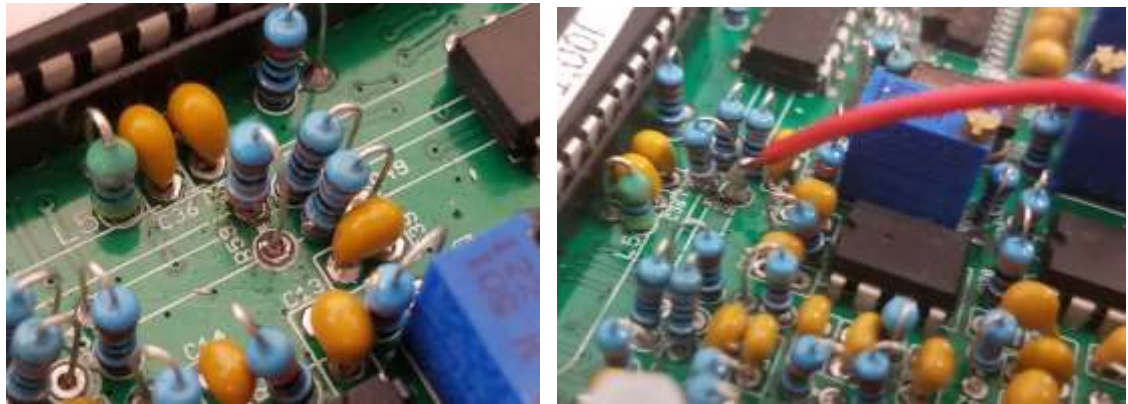
Figure 5: R59 with Orientation Changed (left) and jumper attached (right)
