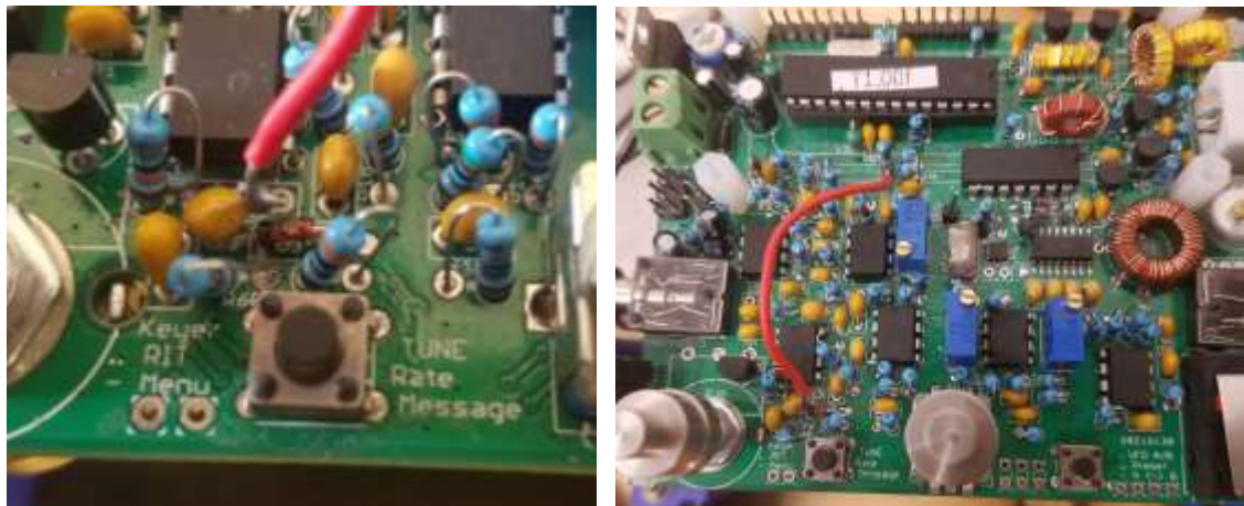
Figure 6: C20 with one end connected to PCB and the wire attached to lead (left) Completed Modification (right)
