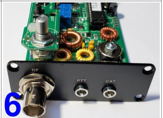
6 Bolt the right-hand side panel to the main PCB using the supplied BNC washer and nut
