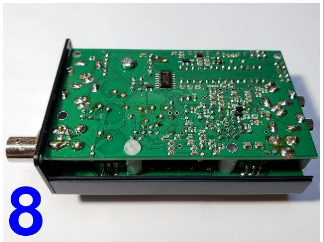
8 Align the 2x5-pin header connector between the main and display boards; some wiggling will be needed to get the controls to fit through the holes in the front panel.
