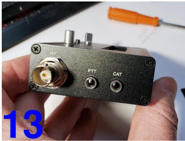
13 Screw in the other four black screws in the corners of the right-hand side panel.
