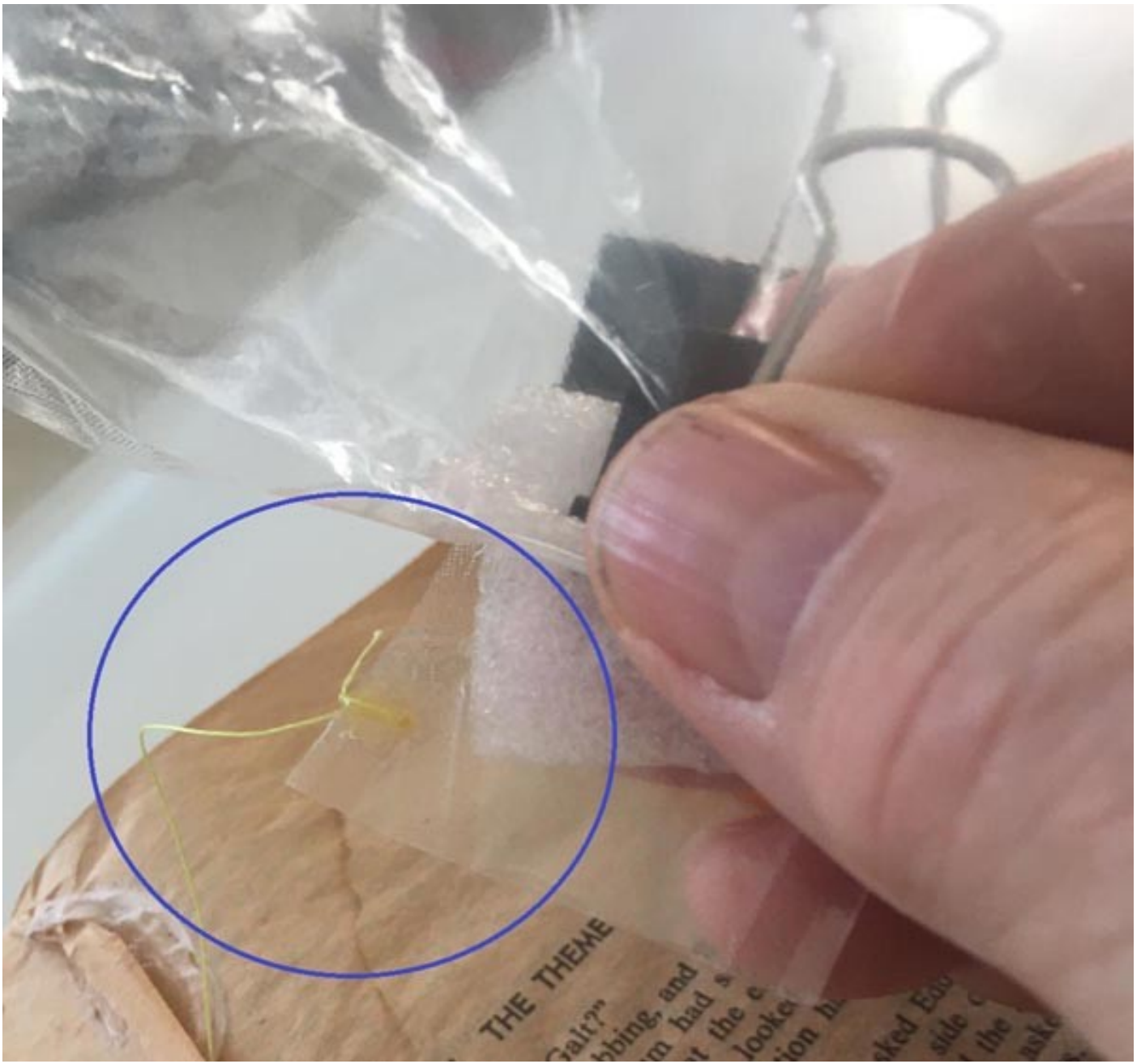
Above Dyneema attachment through a hole in the plastic. Dyneema is tied glued and the hole is glued for strain relief
