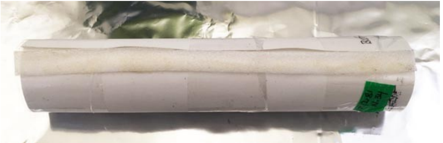
Antenna roll with foam strip to keep wire in tension
