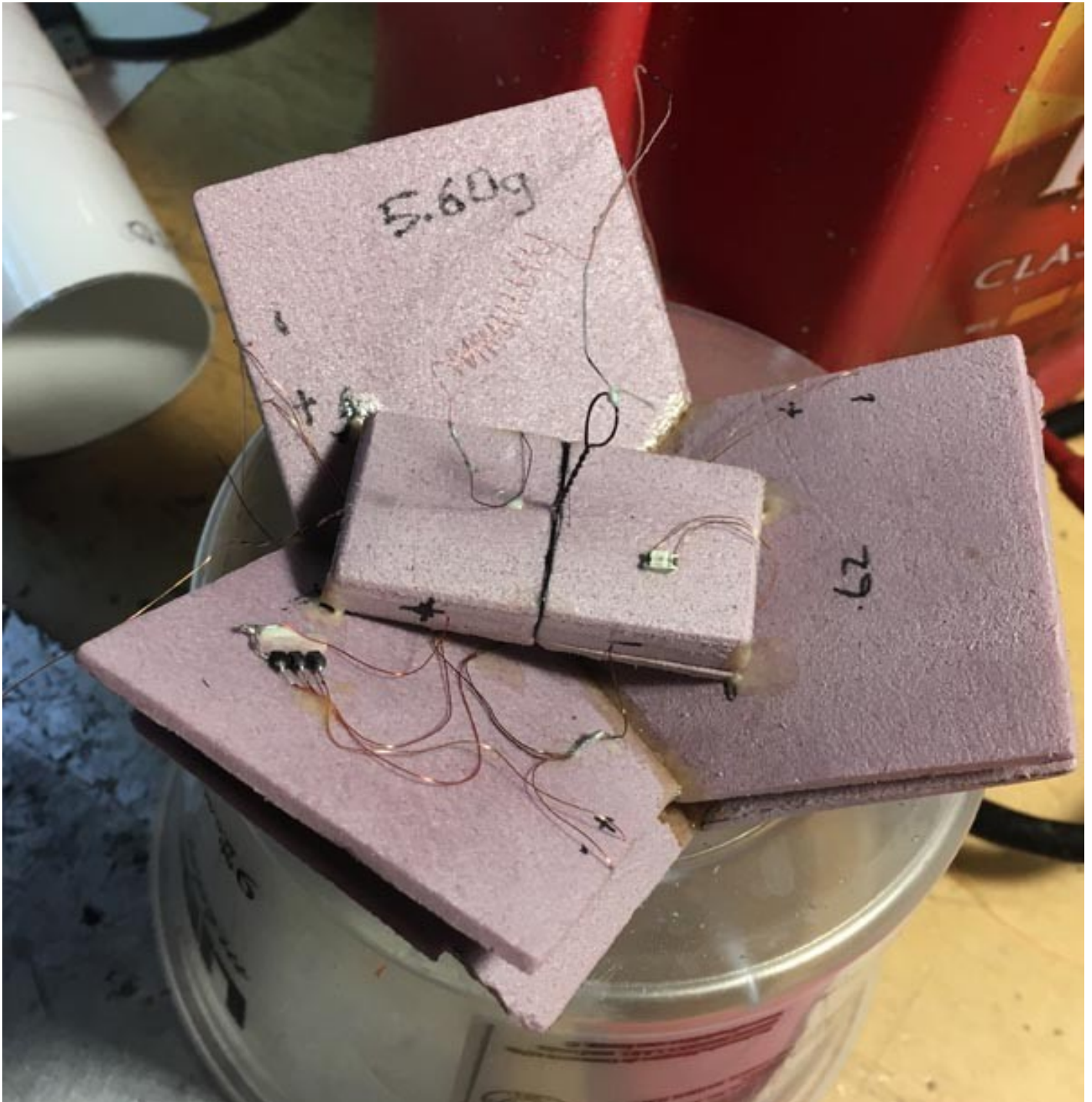
Small coil of antenna wire and soldering detail ..wires glued so they cannot shake loose led downfacing sensor glued down
