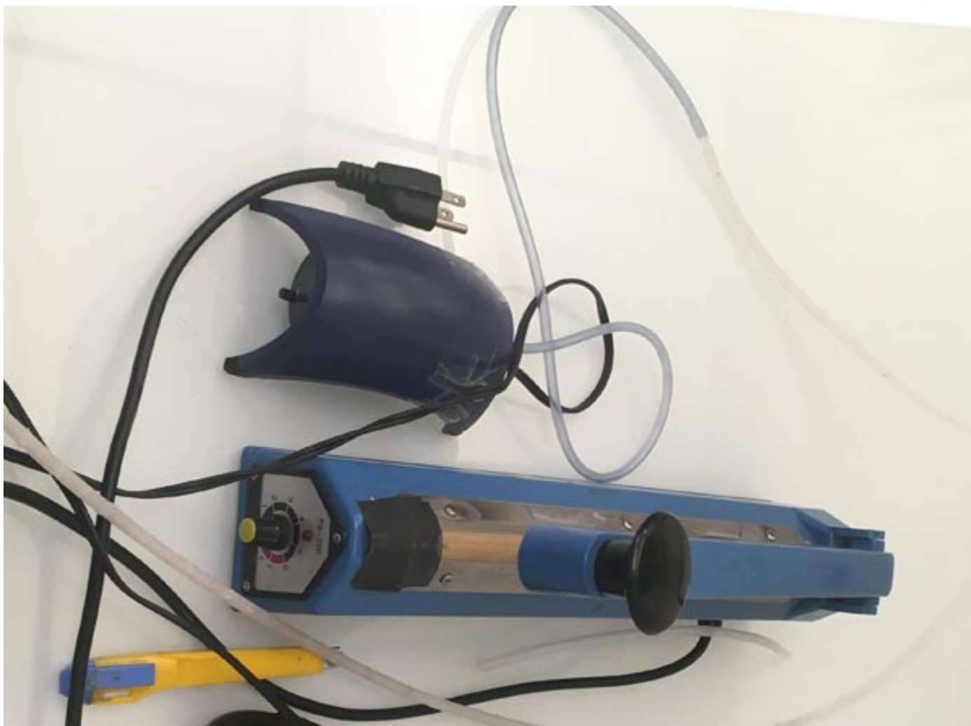
Aquarium pump modified for vacuum and band or impulse sealer with timer for heat control
