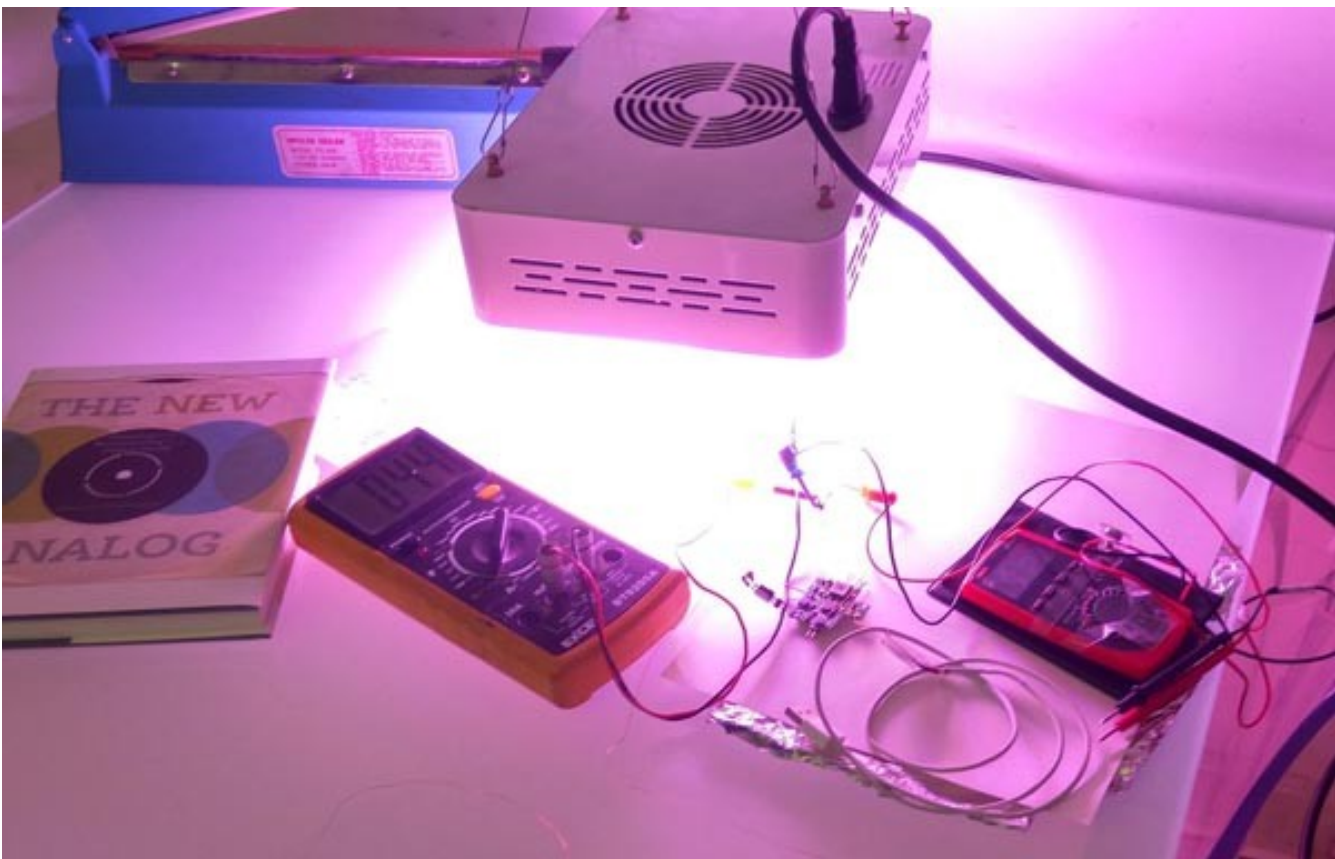
Grow lamp made lots of light to run the solar cells, but also generated too much RFI for the gps to lock
