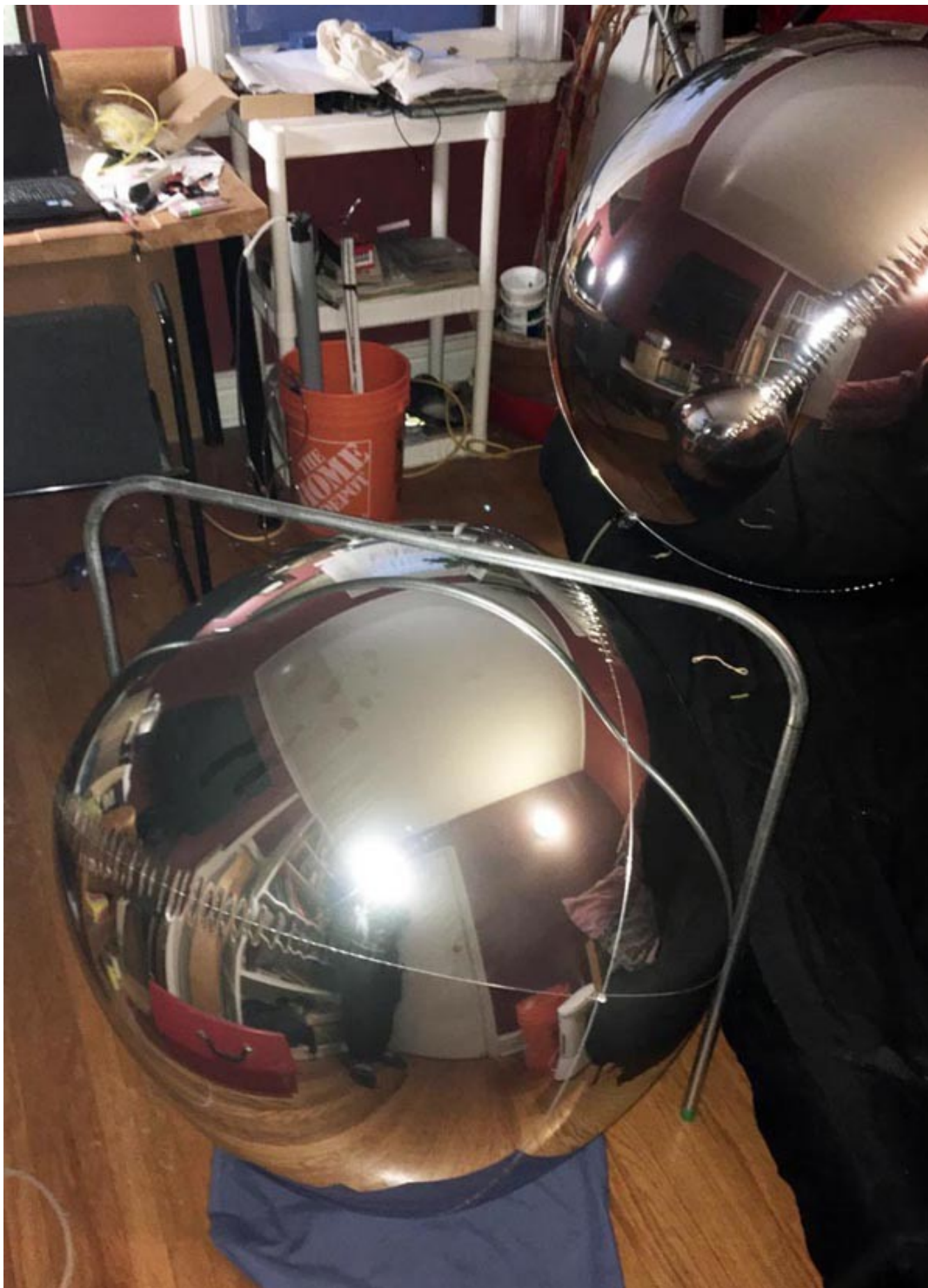
At over 60 percent humidity and .27psi the balloon has reached its design dimensions of 32" and a few wrinkles are visible on the seams but for conservative stretching the pressure was stopped at this volume.
