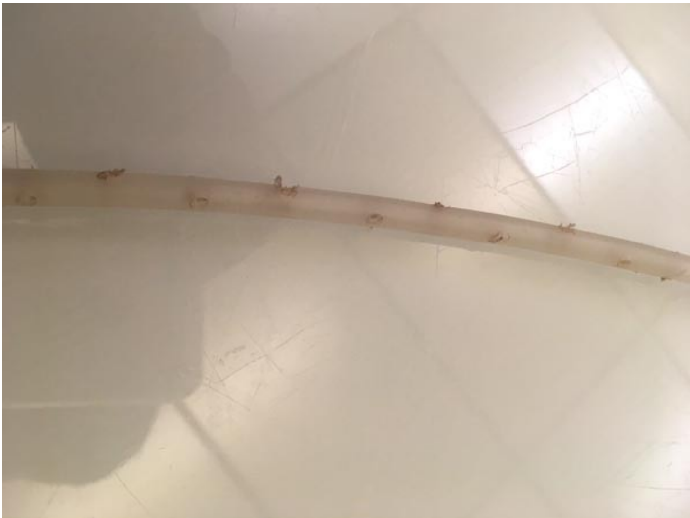
A white plastic tube is drilled in many places and inserted into the balloon to vacuum out the air
