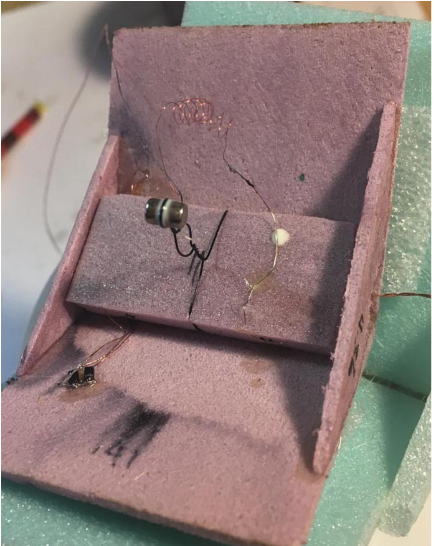
A Neo magnet was used to orient the ridge of the solar collector north and south. Blocking diodes glued down
