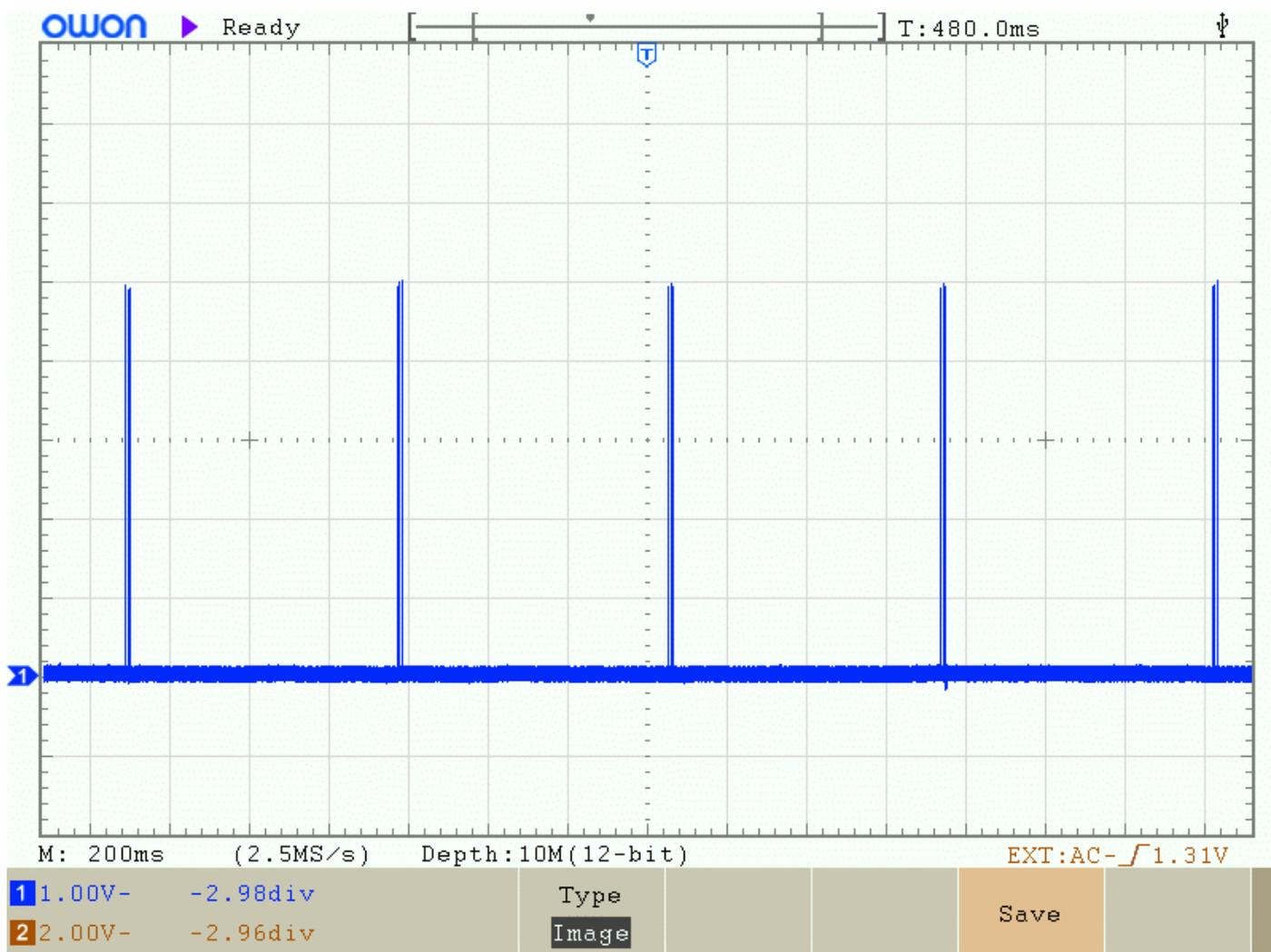
A relay controlled by these outputs will not actually change state due to these short bursts of data. The relay coil simply is slower to react than the duration of the short burst of data. The relay coil cannot de-energise enough for the contact to switch. So the short data bursts are just ignored, as far as the relay is concerned, in this typical use case.
