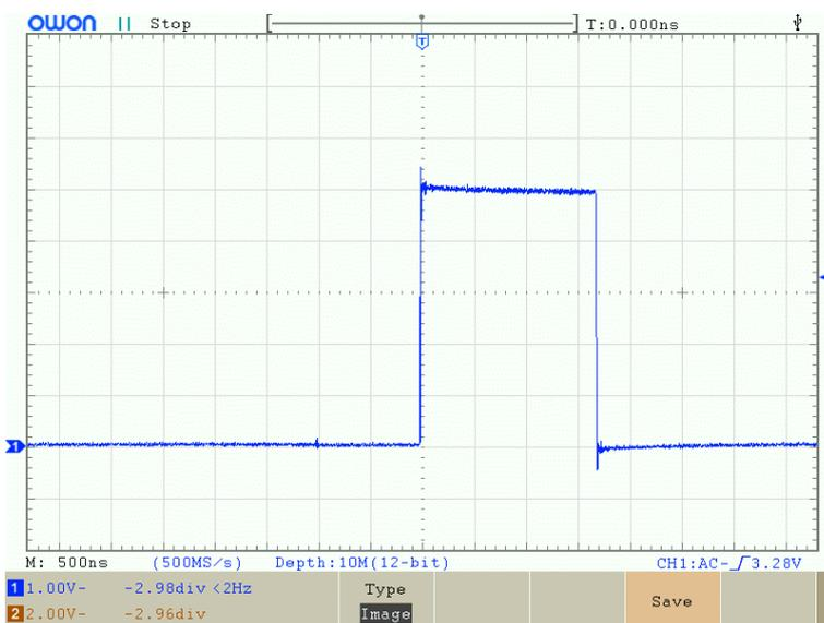
During a WSPR transmission the Ultimate3S kit writes the current symbol transmitted to the display on the bottom row. Again the trace shows the D7 output and D7 is configured to be zero (low). Note the short burst of activity on the D7 signal, which occurs once per WSPR symbol (every 0.68 seconds).
