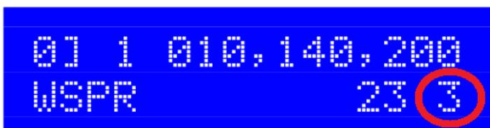
This parameter (3 in this example) is the “Aux” output setting for this transmission screen. It may have the values 0..F. In binary this corresponds to 0000..1111. The value configured here appears on the 4-bit LCD data bus, signals labelled D4..D7 at the edge of the Ultimate3S PCB:
