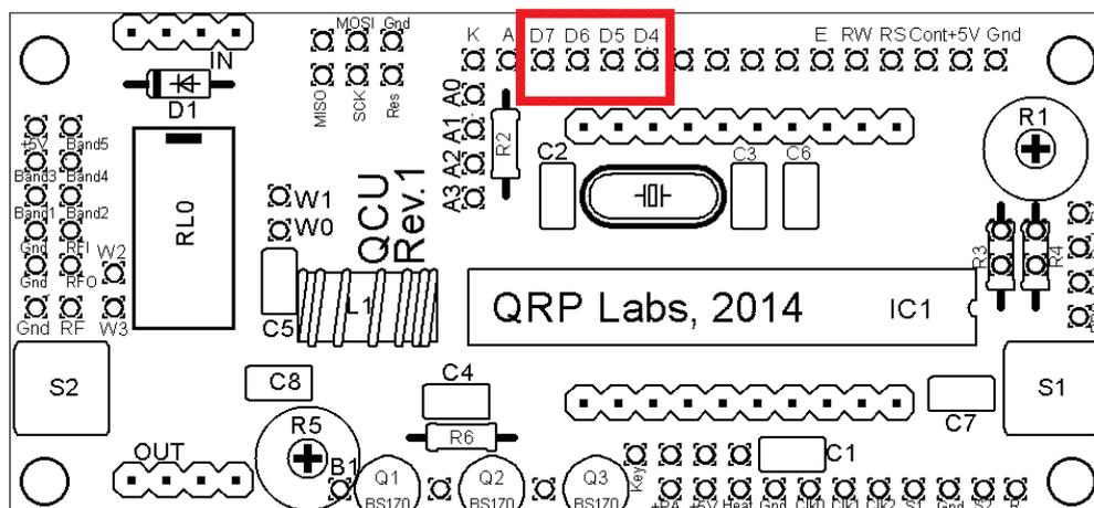
This configuration allows a different value for each of the transmission screens. These four output signals can be used to control external relays, for example.
