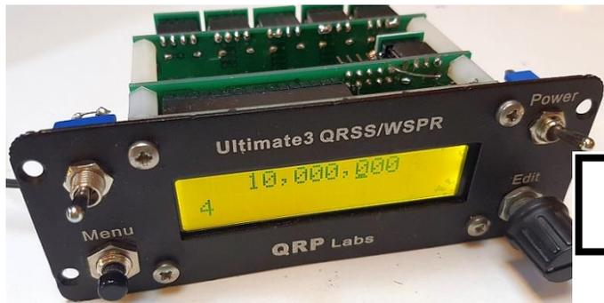
The 60m band LPF filter is plugged into the socket on the main VFO/SigGen board; the other LPFs 40, 30, 20, 15 and 10m are plugged into the relay board. The display is configured simply with the frequency on the top row, and the LPF band slot displayed in the bottom left, using the #LP tag. Here it shows filter 4, which is the position of the 30m LPF used for the displayed 10MHz output frequency.
