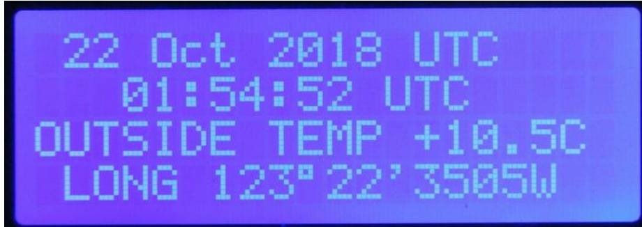
Screen 1: UTC date/time and Outside temperature
