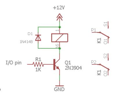
do not omit D1. The supply voltage (12V is shown) should be chosen to match the relay coil used.
