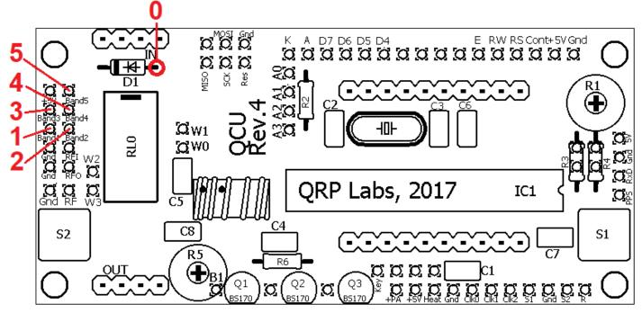
"High" means +5V, "Low" means 0V. You can control whether an output is "Active High" or "Active Low" using the "Active High/Low" character in the alarm display. This is toggled between + (meaning "Active High") and – (meaning "Active Low").
