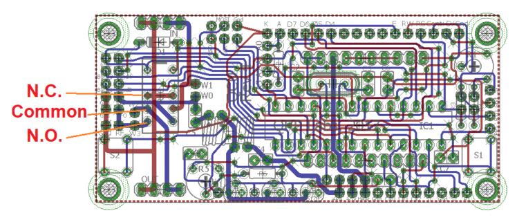
The trace diagram does not show the ground plane which covers the entire top surface of the PCB. It could be difficult to disconnect the N.C. terminals, these are connected to ground. If you wish to use these terminals, you could carefully drill out the through-hole plating from those holes, and use a larger drill bit by hand, to gently remove PCB trace around the hole. Then you could solder wires directly to the relay pin as it protrudes through the PCB.
