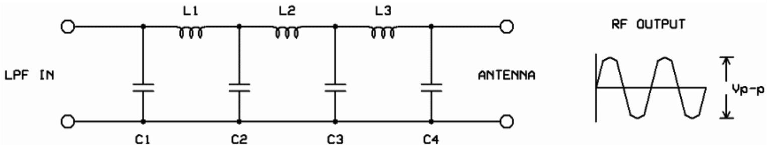
The design uses four capacitors and three inductors wound on toroids, and has 50-ohm input and output impedance. The small PCB has a 4-pin plug at its input and output. It is designed to fit onto the "Ultimate2" multi-mode QRSS/WSPR transmitter kit, but may of course be used as a LPF for other QRP transmitter designs. It also fits the relay-switched LPF kit.
