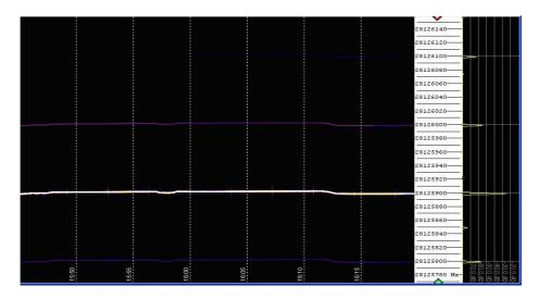
Below see **ocxo\_adjusted2.jpg** after U3 calibration has corrected the output frequency and the OCXO Synth is on long term test.
