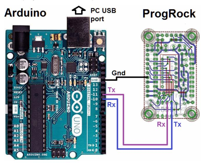
This short example sketch uses the Arduino SoftwareSerial library. Both ports are run at 9,600 baud. Received serial data on either input is re-transmitted to the other output.
