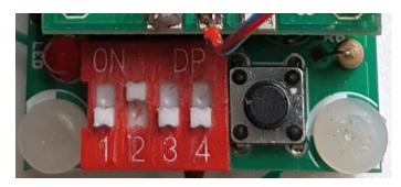
Start-up switch positions for serial port configuration
