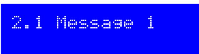
Turn the rotary encoder to select the Message from 1 to 12 which you wish to edit, then press the left (“select”) button. Now you can edit the message text in one of two ways:
