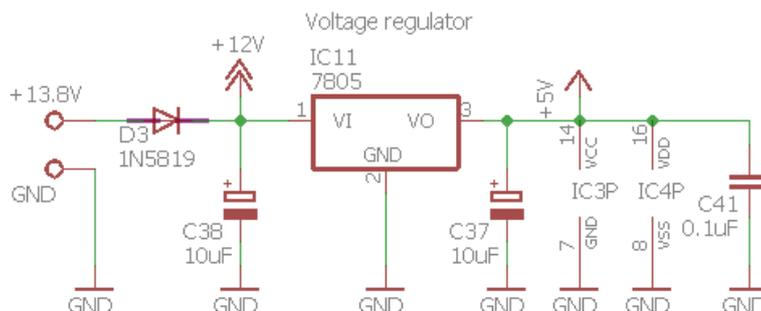
If you are brave, and confident that you will NEVER connect power to the radio with reversed polarity, you can omit this diode and fit a jumper wire over it.
