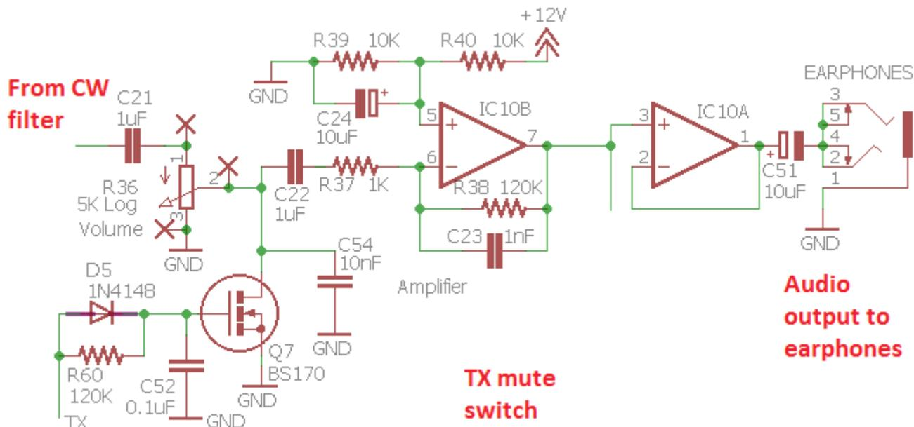
There is also a TX mute switch formed by Q7, another BS170 MOSFET. This was a late addition to the design: despite all attempts, I could not remove the nasty click on receive/transmit switching. The mute switch helps to attenuate it. The switch is operated by the microcontroller Receive/Transmit switch output. When the BS170 switch is on, it has a low resistance to ground which greatly attenuates the audio signal.
