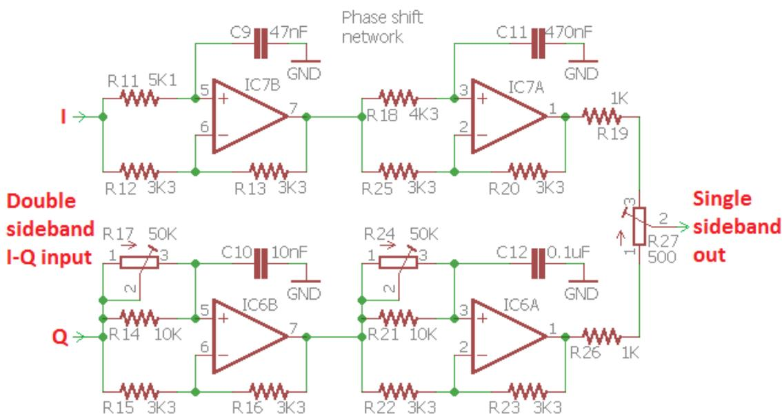
By this stage the I and Q outputs are each double-sideband, and we need to process them to demodulate single sideband.
