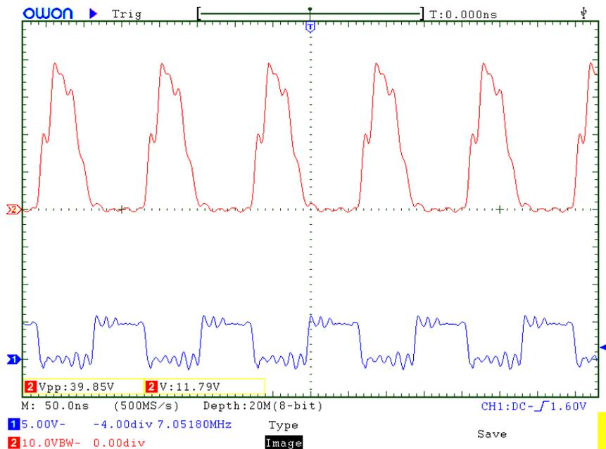
The important point to note is that when the BS170 are switched ON (the gate voltage is 5V), the drain voltage is zero. When the BS170 is OFF the gate voltage pulses nicely to a large amplitude. Class-E!
