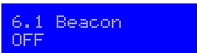
This is the master switch controlling whether beacon mode is enabled or not. If beacon mode is enabled, then the radio starts operating in beacon mode on power-up.
