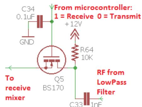
The transmit/receive switch is implemented by a single BS170 MOSFET. The source is at DC ground (via the primary of input transformer T1). The control signal from the microcontroller switches the MOSFET on or off. Interestingly, capacitor C34 close to the MOSFET gate is found to be necessary to prevent inductive pickup of the 5W RF from partially switching on the MOSFET.
