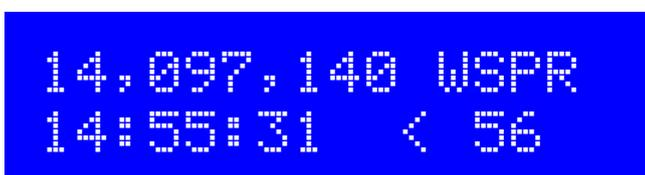
When a GPS unit is connected, the firmware automatically uses the 1 pulse-per-second signal to measure the transmit frequency and compensate for any inaccuracy due to calibration error or frequency drift due to temperature. The serial data stream from the GPS is used to set the real time clock (for syncing the WSPR transmission timing). The Maidenhead locator is computed from the latitude and longitude information parsed from the GPS serial data.
