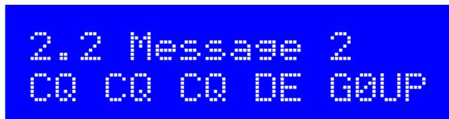
By far the easiest way to edit TEXT parameters is simply to use the CW decoder! As before, it expects well-timed CW, with correct spacing between words and characters. The CW decoder expects you to key in the characters at near to the configured Keyer speed. If you start keying at a much different speed, the CW decoder will adapt to your keying but this may take several characters to “sense” your keying speed, so some characters can be missed.
