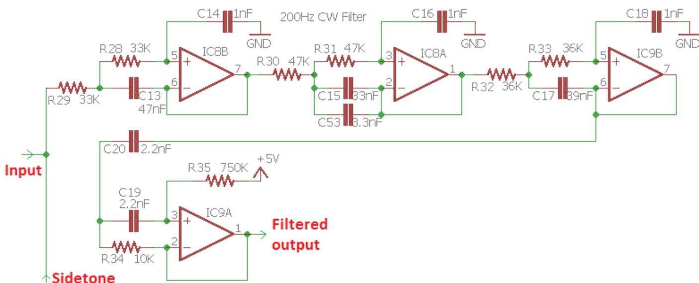
There are three stages of low-pass filtering and one stage of high-pass filtering. The first three stages retain the 2.5V “midrail” bias all the way through from the input transformer T1. The final stage IC9A is biased using the 5V supply (avoiding a few extra components to create a real 6V mid-rail at half the supply).
