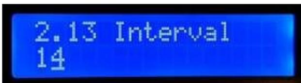
The underline cursor below the 4 indicates that editing is active; turning the rotary encoder will change the parameter value.
