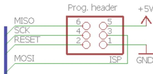
The ISP interface uses the same I/O pins as the GPS interface and the Paddle. When upgrading the firmware, be sure to disconnect the GPS (if you had one connected). And do not press any paddle key while doing the firmware update!
