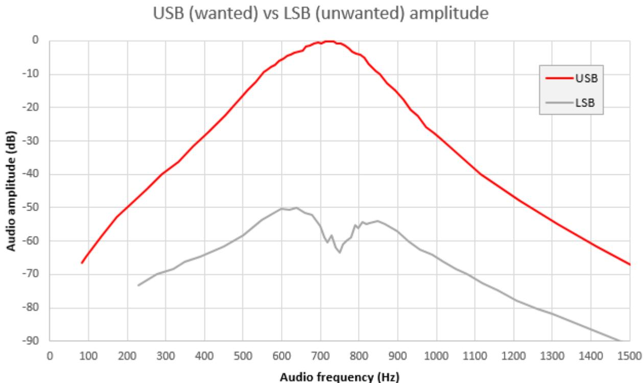
Subtraction of these two curves results in the unwanted sideband level as shown in the following chart. Normally anything above 40dB rejection is considered good; above 50dB is excellent. With the built-in adjustment features of this kit it is relatively easy to achieve really excellent unwanted sideband rejection.
