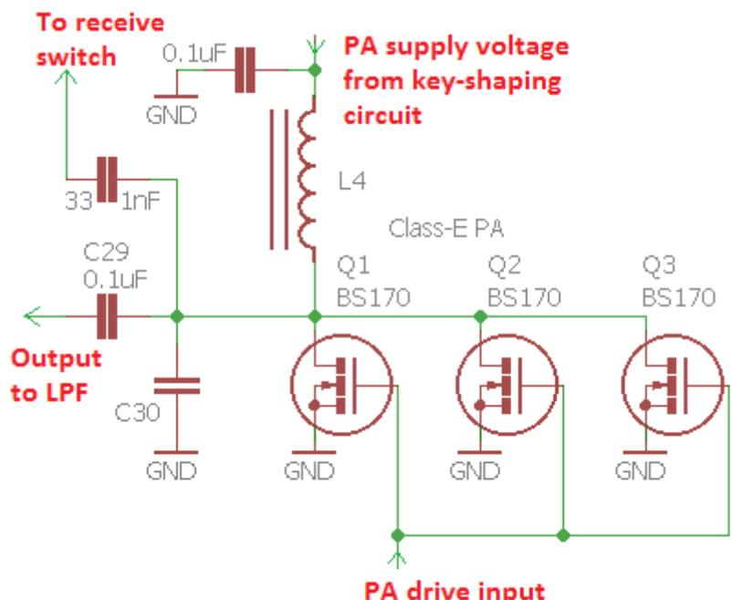
A Class-E Power Amplifier contains a resonant circuit at the frequency of operation, so it is only suitable for single-band use. A lot has been written about Class-E, much of it is very technical and mathematical.
