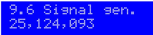
The signal generator function is switched off until you press the left button to select it. Then the cursor appears under the 10MHz digit. You can then adjust this number just like any other configuration parameter. Use the rotary encoder to increase or decrease the frequency. Press-and hold, then turn the rotary encoder, to change the tune rate (move the cursor left or right).
