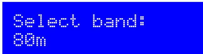
Turn the rotary encoder knob to select the band you have built the kit for. Then press the small button to the left of the rotary encoder, to make your selection.
