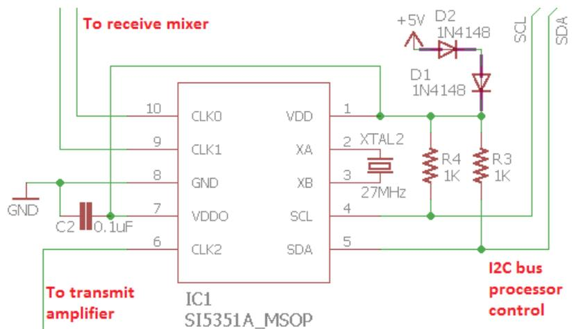
The Si5351A has a large number of internal 8-bit registers to control the synthesiser behaviour, and these are programmed by the microcontroller using the I2C serial protocol. 1K resistors R3 and R4 are pull-ups required for the operation of the bus at 400kHz.
