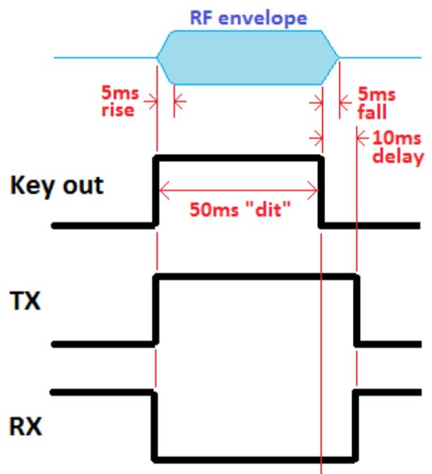
The “TX” signal is the inverse of the “RX” signal, and it switches the gate of the audio mute switch Q7 during transmit. One of the NAND gates IC3D is used as the inverter to create the “TX” signal from the microcontroller’s “RX” output.
