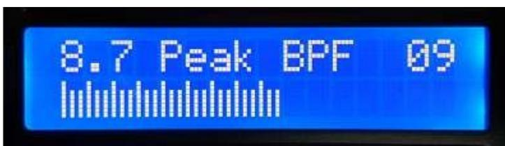
Adjustment of the C1 trimmer capacitor should change the size of the amplitude bar. You need to adjust the C1 trimmer for MAXIMUM amplitude. When this is done, the peak of the band pass filter will be centred on the CW section of the band.
