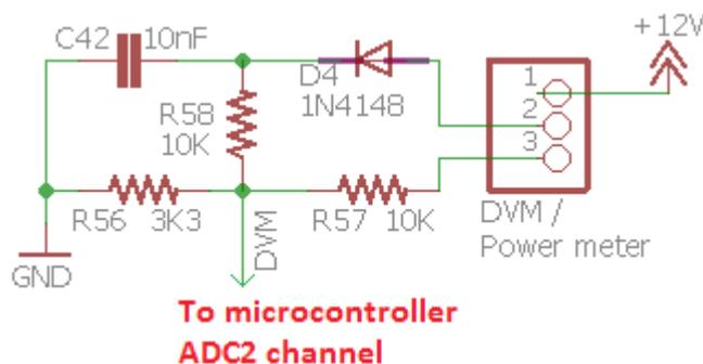
When measuring RF power, connect the RF to be measured to pin 2 of the 3-pin DVM/RF Power connector. In this case D4 and C42 form a simple RF detector. The RF is rectified by D4 and smoothed by C42. R56 (3.3K) and R58 (10K) again form a potential divider that divides the rectified voltage by a factor of 4.03. The resulting range of the power meter is from 0 to 5W approximately.
