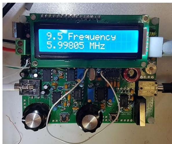
shown here in the photograph (right); clearly the 2kHz low reading indicates I have not calibrated the 27MHz reference value and/or the 20MHz system clock value!
