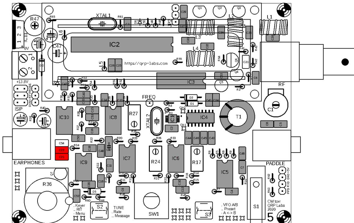
Note that C54 is an optional capacitor that \*may\* improve the Rx/Tx changeover “click”. It is not supplied, do not fit it initially. You may wish to experiment with it later. In subsequent sections this capacitor is shown shaded GREY; you have not installed it, but you are not going to install it.
