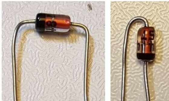
In all cases it is critical to install the diodes the right way around, these are a polarised component and must only be installed in the PCB with the correct orientation! In the case of D1, D2 and D5, the PCB silkscreen printing shows a white stripe at the end of the diode body which must match the black stripe on the left end of the diode (photo above).
