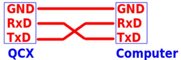
Remember QCX RxD connects to the computer TxD, and the QCX TxD connects to the computer RxD; there is a swap as shown. Most PCs do not have actual serial ports anymore and the typical set-up will be to use a USB to Serial converter. **Be sure to use one with TTL level serial data, NOT RS232 which is a different (higher) voltage.**
