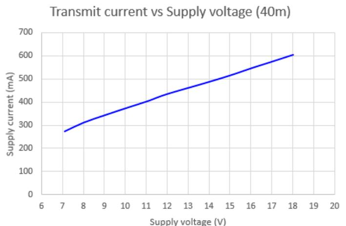
At supply voltages above 13.8V, check the temperature of the 7805 voltage regulator, which may need a heatsink as it dissipates more heat at higher supply voltages.
