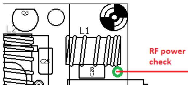
At the top right corner of the PCB, you will find a pad on the PCB where the L1 wire is soldered in. This pad is connected directly to the RF output pin of the BNC connector (see diagram). If you connect a wire from here, to pin 2 of the 3-pin DVM/RF Power header, then key-down, the display will read the power output in Watts. It is easiest to have the transceiver in Straight key mode and just press the microswitch.
