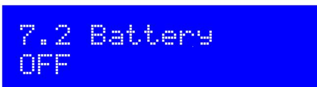
This BOOLEAN parameter controls whether or not the battery icon is displayed on the screen at the top right corner. Measurement and display of battery voltage may be useful to those operators who intend to operate the radio from battery power, for example during portable operations.
