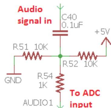
The ADCs in the ATmega328P have 10-bit resolution which translates to about 5mV. The ADC conversion result is a number in the range 0-1023, with 512 representing zero. An audio voltage of
