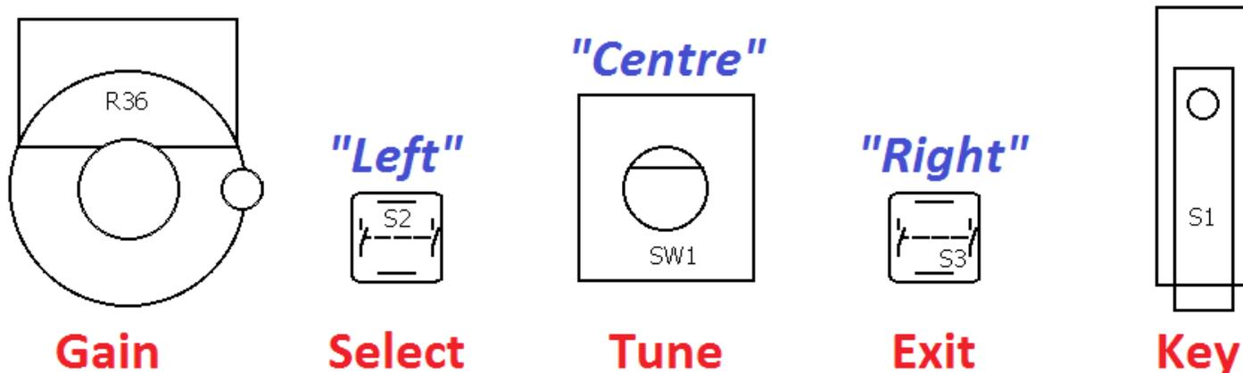
This diagram shows the operating controls of the radio. All of the controls except the Gain potentiometer have multiple functions, depending on the operating mode, menu editing, etc. The tuning rotary encoder in the centre has a button on its shaft that is activated by pressing it, and this button also has multiple functions.
