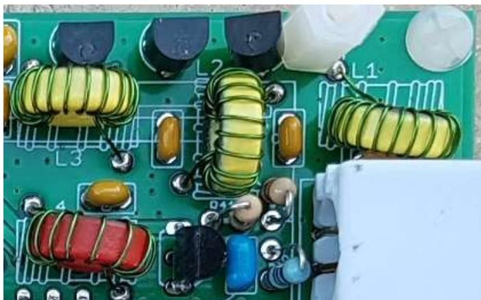
Insert the ends of the wires into the correct holes of the PCB and pull it through tight, so that the toroid sits up vertically on the PCB. See photo, right.
