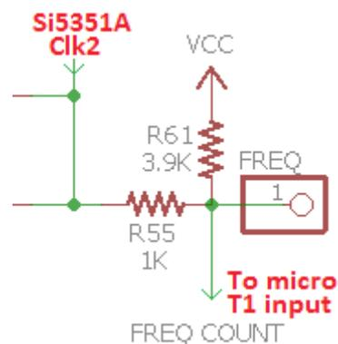
Since the 3.3V peak-peak signal from the Si5351A is rather marginal for operating the Timer1 input, a 3.9K pullup resistor increases its centre point. Now “low” is 1.02V and “high” is 3.65V, which is enough to trigger the Timer1 input reliably.
