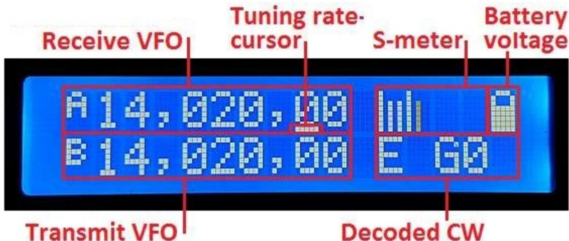
The main display layout during ordinary operation (which will be called “main operating mode”) is shown in the above photograph. The display during beacon or message transmission modes, menu editing, alignment etc. differs. The main display elements are as follows:
