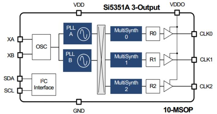
For best jitter performance, the Si5351A datasheet recommends the use of even integer dividers (no fractional component) in the MultiSynth dividers and in this CW transceiver design, this recommendation is followed.
