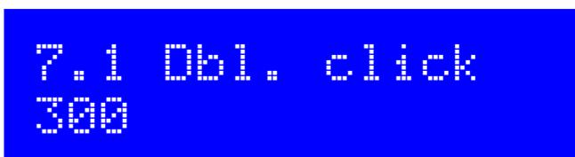
This is a NUMBER parameter which controls the decisions on what type of press has been made to a button. By default, it is set to 300 milliseconds (as shown here) but you may alter this if you wish.
