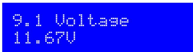
This is the Digital Voltmeter (DVM) function. The measurable voltage range is 0-20V DC.
