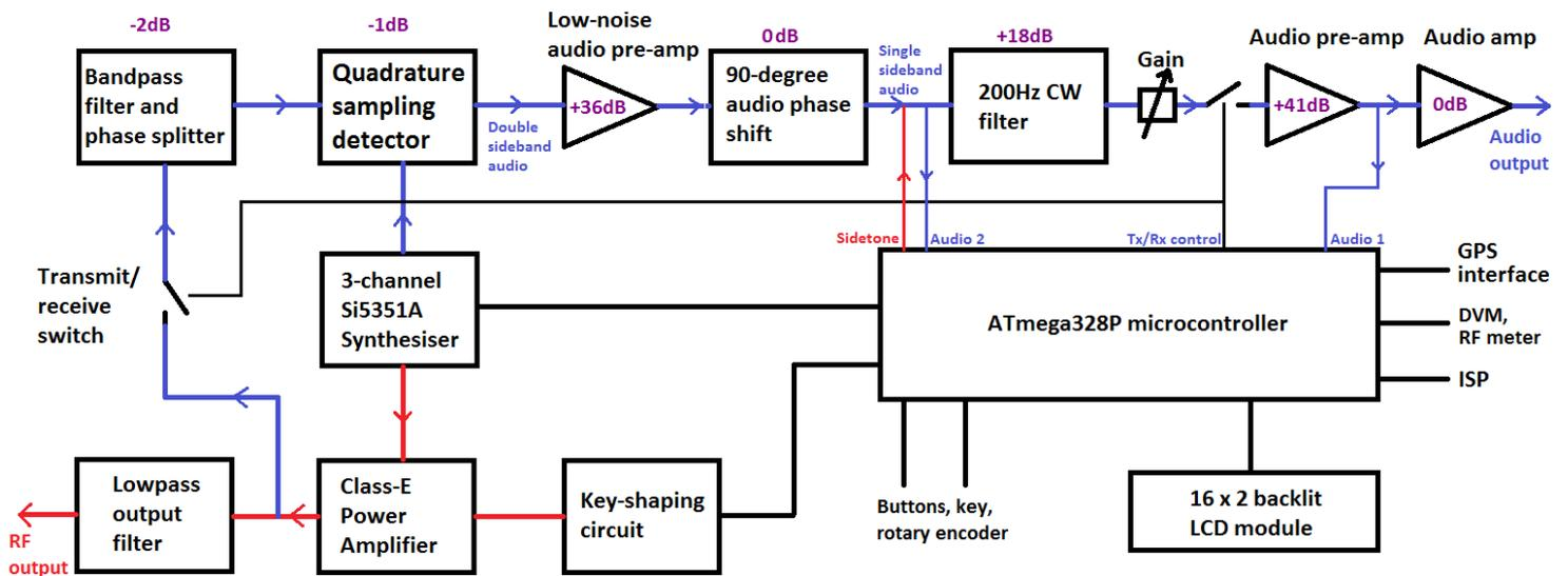
This CW transceiver is a high performance, yet simple and low cost, analogue design. The transmitter uses a high efficiency Class-E amplifier which results in low current draw on transmit, and inexpensive transistors with no heatsinks.
