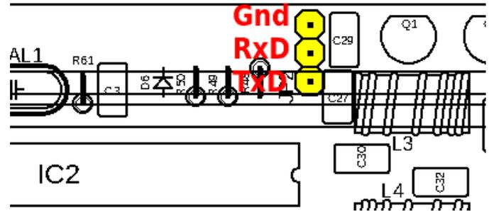
The three pads (GND, RxD, TxD) are not conveniently located near the board edge, and a 3-pin header on the upper side of the board could not be used because it would conflict with the LCD module plugged in here. This non-ideal location of the three pads is because the CAT interface was added relatively recently in the QCX design evolution.
