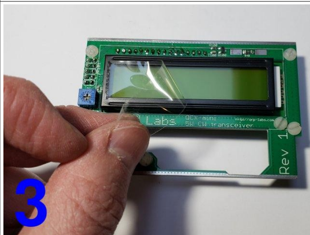
3 Peel off the plastic protective coating from the LCD module.
