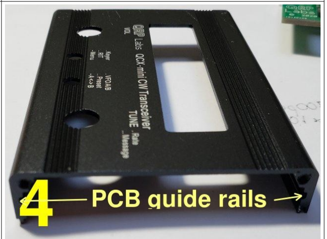
Here's the top half of the enclosure. Note the PCB guide rails in the extrusion walls.
