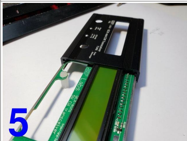
Slide the display board into position along the PCB guide rails in the enclosure.
