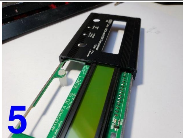
5 Slide the display board into position along the PCB guide rails in the enclosure.
