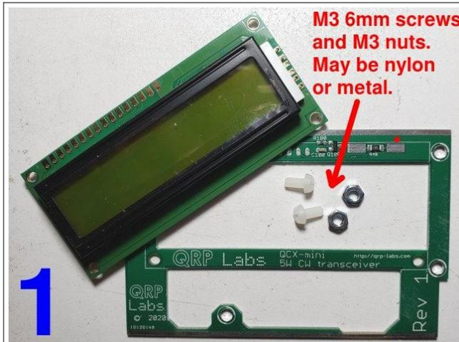
Identify the pairs of M3 6mm screws and nuts. They may be nylon or metal.
