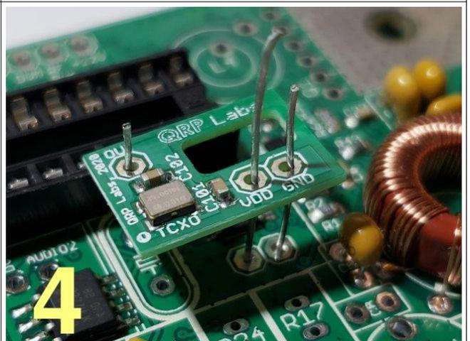
Thread the TCXO module carefully onto the wires. Make sure module is pushed as far
