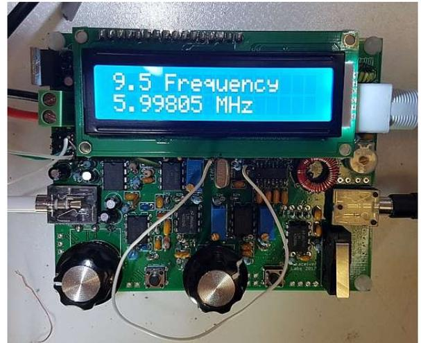
In the photograph, the white wire shown looping around the rotary encoder connects the FREQ pin (just under the “M” character of the LCD, in the photograph) to the Clk0 output pin (just under the “z” character of the LCD).
