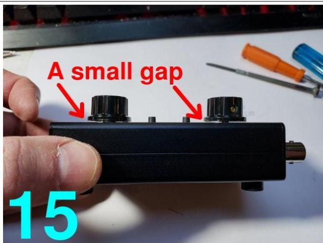
Install the supplied knobs by tightening their grub screws. Leave a small gap between each knob and the front panel, to allow the knob to turn easily. The grub screw of the volume control knob should be at the position of the flat on the shaft. The grub screw position on the rotary encoder is not important.
