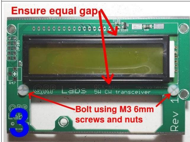
Bolt the LCD module, ensuring equal gaps at top and bottom; tighten screws firmly.
