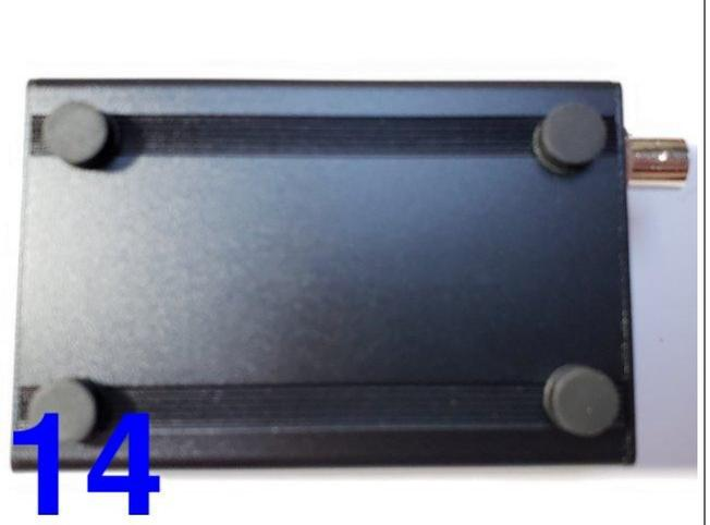
Apply the supplied four self-adhesive feet to suitable positions on the base of the enclosure if desired (optional).
