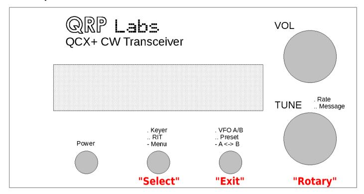
This diagram shows the operating controls of the QCX+ radio as an example. All of the controls except the Gain potentiometer have multiple functions, depending on the operating mode, menu editing, etc. The tuning rotary encoder at the bottom right has a button on its shaft that is activated by pressing it, and this button also has multiple functions.
