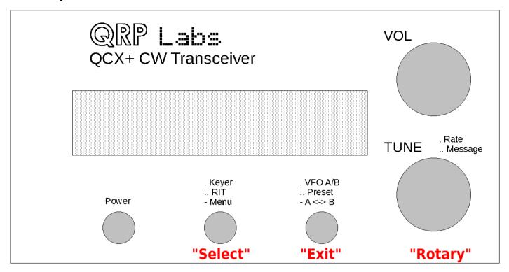
This diagram shows the operating controls of the QCX+ radio as an example. All of the controls except the Gain potentiometer have multiple functions, depending on the operating mode, menu editing, etc. The tuning rotary encoder at the bottom right has a button on its shaft that is activated by pressing it, and this button also has multiple functions.
