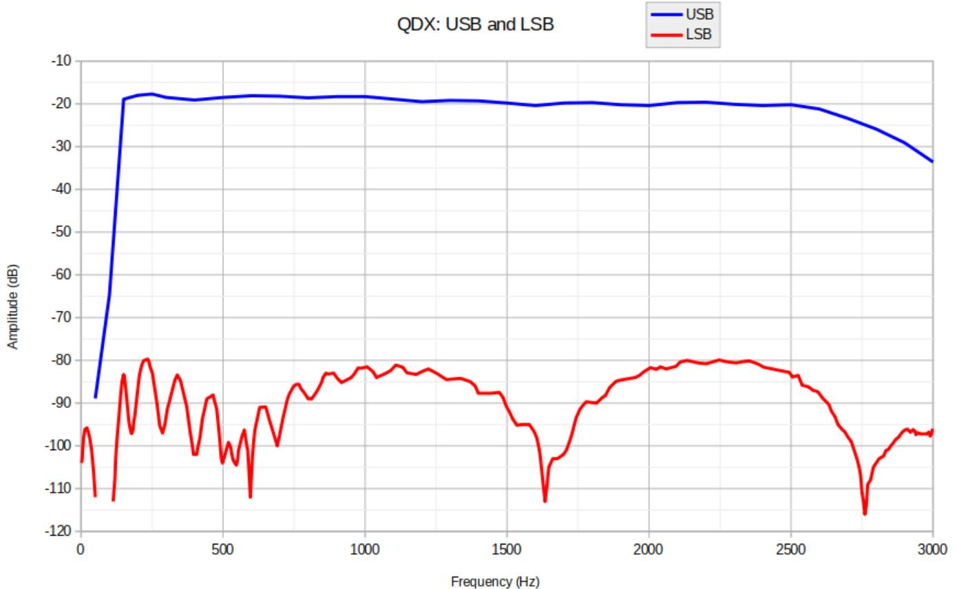
Despite no attempt to correct for errors, the unwanted sideband suppression is still an impressive -60dB in this example. There will naturally be some variation from unit to unit.
