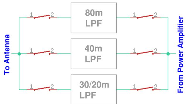
The filters were designed using the freeware Elsie program by Tonne software (<http://tonnesoftware.com/elsie.html>). The filter topology is a 5-element filter, with a 6<sup>th</sup> (capacitor) creating a resonant trap. For the 80 and 40m filters, the design was optimized to satisfy the following criteria:
