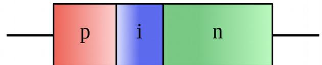
fast enough to rectify RF. PIN diodes can be expensive components and hard to find. But luckily, the common 1N4007 diode, with its 1,000V PIV rating, happens to have a type of construction resembling a PIN diode, and operates very well as a poor-man's PIN diode, from the 630m band to the 10m band inclusive.
