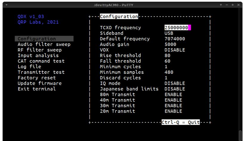
Transmit can also be enabled by band, this could be useful to prevent accidental transmission into high SWR on bands your antenna isn't optimized for.
