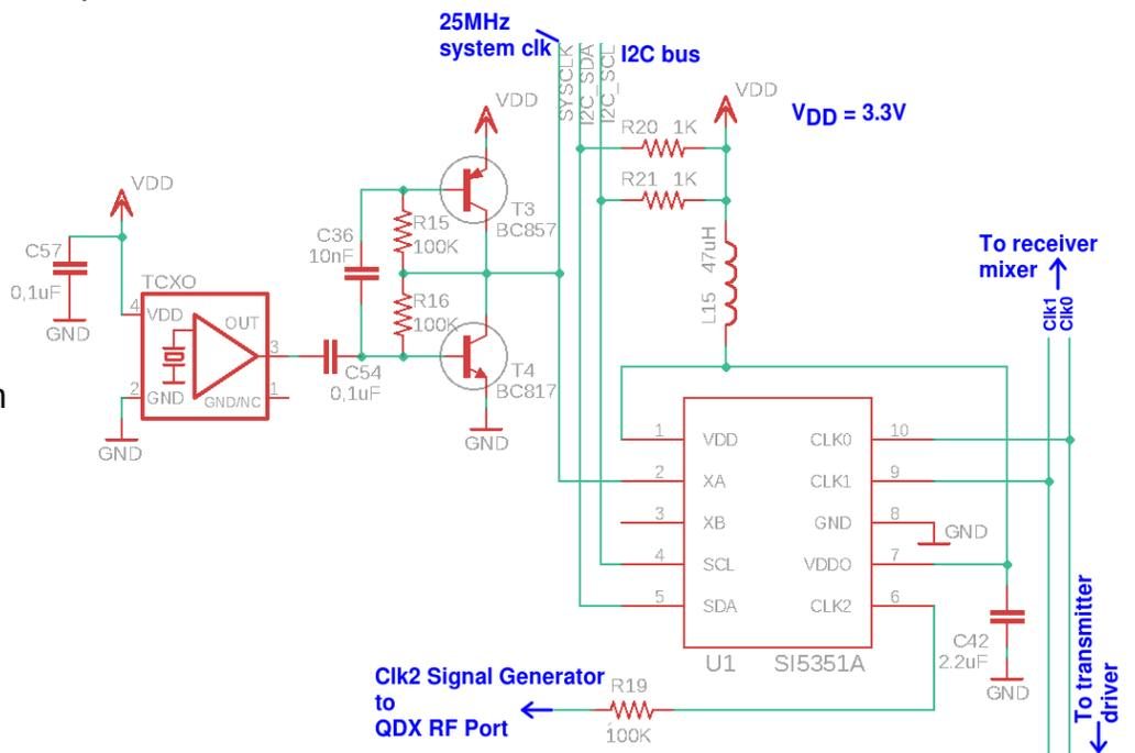
also used to clock the microcontroller. The reason for this is that it is a very good design rule, to try to minimize the number of different oscillators in a radio design – harmonics of oscillators somehow find a way to mix and create receiver birdies.
