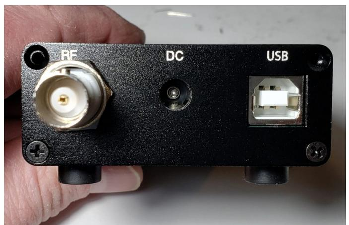
On the front panel is a single solitary status LED, and on the rear you'll find just three connectors: RF (BNC connector for the antenna), DC power in, and a full-size USB B connector. The Rev 3 PCB also has a 3.5mm jack socket as a configurable PTT output to activate an external amplifier. Let's not talk more about such QRO matters in polite QRP company.
