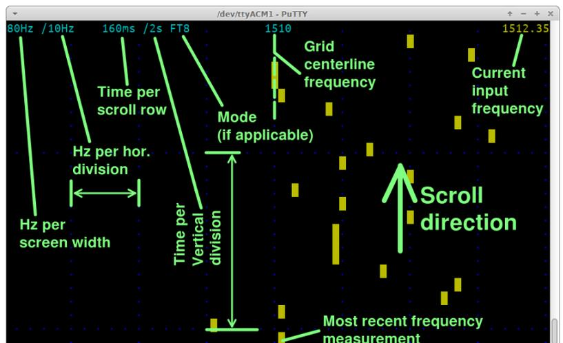
This example shows FT8, the screen scrolls every 160ms which is the FT8 symbol rate, and the screen bandwidth is 80Hz which is sufficient to show all the tone symbols of FT8's 50Hz bandwidth.
