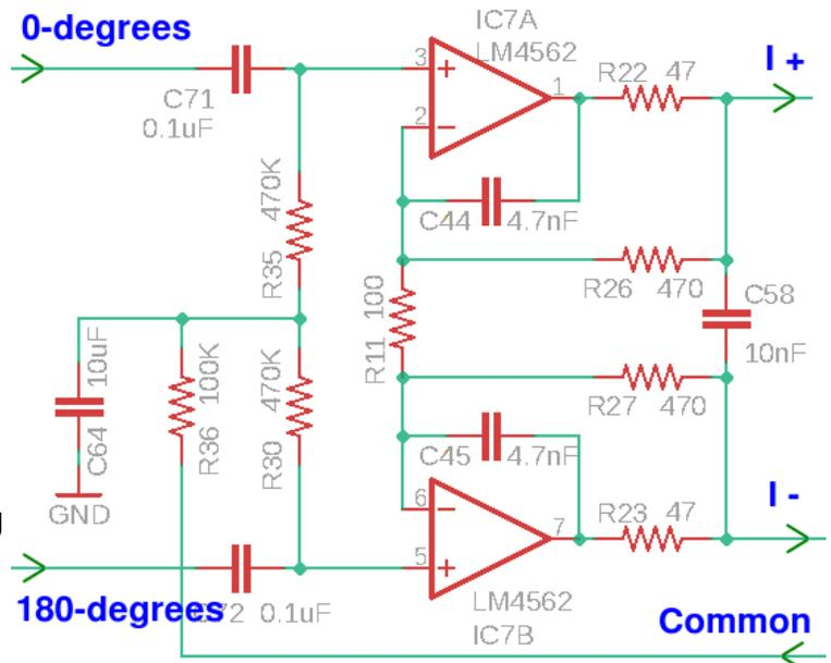
Differential amplifier ICs are available but expensive, and less commonly available parts. It is preferable to assemble a differential amplifier from normal operational amplifiers. The LM4562 has been a QRP Labs favourite, offering a good balance between performance (low noise) and price.
