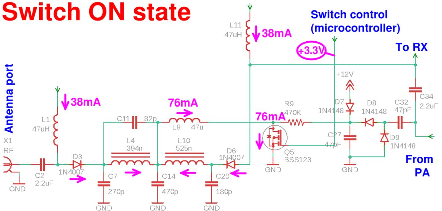
The 3.3V (logic "1") signal from the microcontroller switches on Q5, which then pulls down the center point of the Low Pass Filter via inductor L9. Forward bias current flows from the bias control circuit through L1 and L11, passing about 38mA through each diode (assuming 12V supply).
