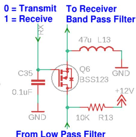
The transmit/receive switch circuit is very simple, just a MOSFET that is switched ON to allow signals to reach the receiver, and OFF to block them. Nothing more than that is needed.
