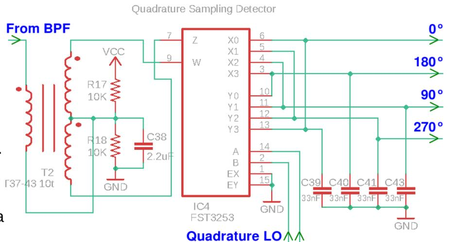
T2 is a trifilar transformer that efficiently splits the signal into two 180-degrees out of phase signals for the detector (IC4). The integrating capacitors C39/40/41 and 43 at the four outputs need a lower value of capacitance for higher bandwidths. QDX samples baseband at 48ksps and 33nF was determined to be a good and appropriate value for this bandwidth.
