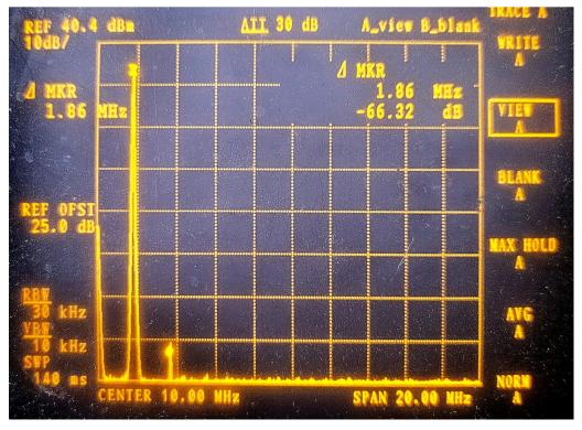
For testing the Receiver section, use the RF Sweep tool in the terminal. Use the + - keys to go up a band (though other bands are not enabled) then go back to 160m; this is because the first RF sweep in the tool has a firmware bug which causes inaccurate results. There should be a peak somewhere near the band center frequency (indicated by the vertical dashed line) as shown below. It isn't terribly critical if the peak occurs a bit to the right or left of this.
