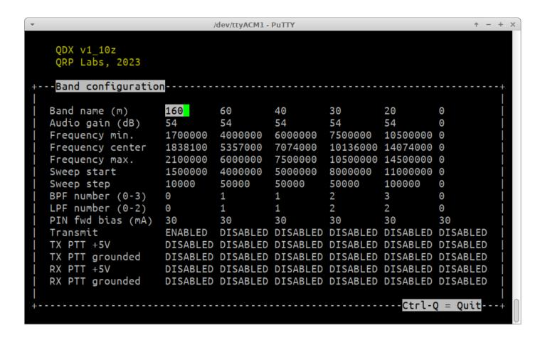
The BPF number, LPF number and PIN fwd bias cells have no meaning for the QDX-M because it is single band and there is no band switching. So you can ignore those. It is a very good idea to set the "Transmit" cells for all the other listed bands to "DISABLED" to prevent any accidental mishaps trying to transmit at incorrect frequencies into the 160m Low Pass Filter of your QDX-M.
