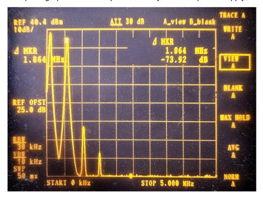
For testing the Receiver section, use the RF Sweep tool in the terminal. Use the + - keys to go up a band (though other bands are not enabled) then go back to 630m; this is because the first RF sweep in the tool has a firmware bug which causes inaccurate results. There should be a peak somewhere near the band center frequency (indicated by the vertical dashed line) as shown below. It isn't terribly critical if the peak occurs a bit to the right or left of this.
