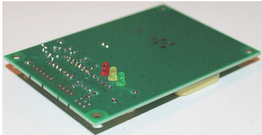
This photograph shows the usual method of assembly, with the LED’s on the solder-side of the PCB so that with the patch antenna installed on-board, they’ll be visible.
