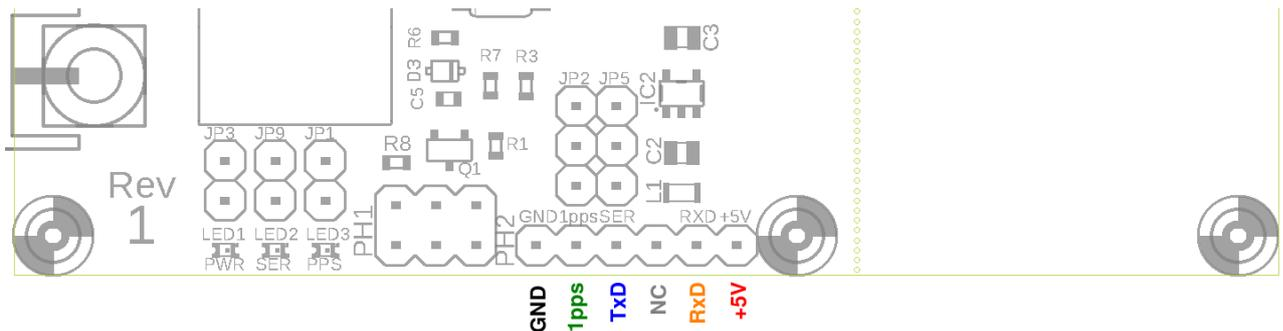
The 1pps, Serial data, TXD and RXD signals can be configured to be either 2.8V/3.3V logic level, or 5V logic level. The configuration is done using jumper wires that will be described in the next section. Note that 2.8V logic will be compatible with 3.3V systems, without issue.
