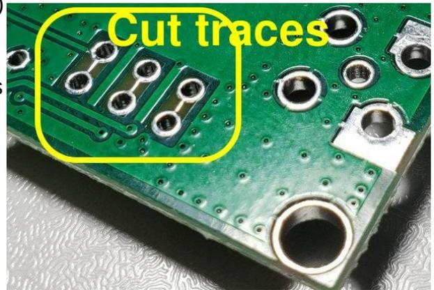
You would also need to cut the thin exposed tinned copper traces on the underside of the PCB, in order to disconnect the onboard LEDs. This should be done with a sharp knife, carefully so as not to damage any other nearby traces.
