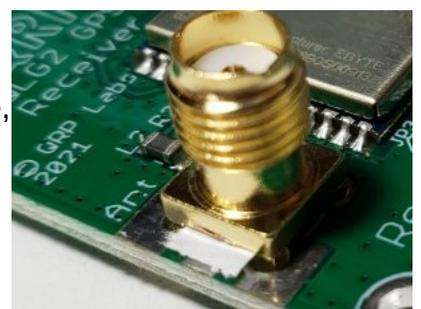
**Horizontal installation:** The SMA connector happens to fit the board nicely too in the horizontal, edge-mounted position. Place it with the center pin on the top side of the board, and two of the corner pins on the bottom side, and solder in place. The other two ground pins can be ignored. This works very well.
