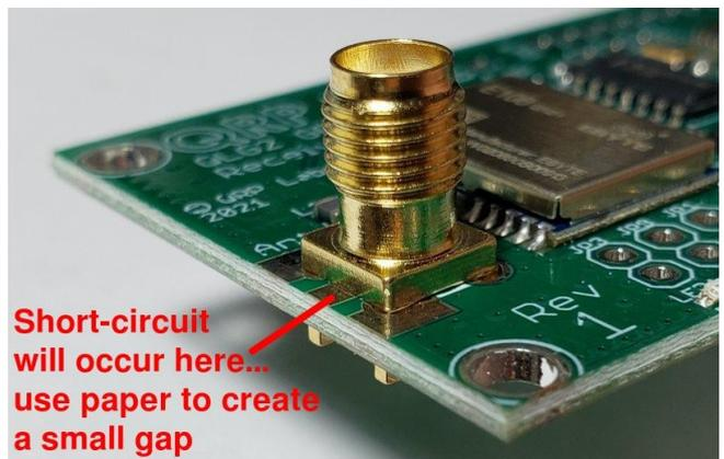
**Vertical installation: IMPORTANT! The body of the SMA connector WILL DEFINITELY short to the center pad of the component footprint on the board.** This will not only short out the antenna, rendering it completely ineffective, it will also draw high current from the GNSS module through the 10-ohm resistor R2. You will soon note the temperature rise of the GNSS module as well as the 3.3V voltage regulator chip (you don't need to ask me how I know...).
