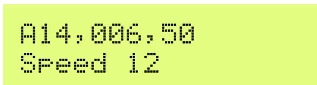
Now you can adjust the speed using the rotary encoder. Press any button to return to the main operating mode. You may operate the radio while the Speed setting is shown. You can also press the rotary encoder shaft button to select sending a stored message, while the Speed adjustment setting is active.
