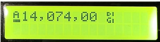
Everything is fine! TX state, enough audio, and so you should have RF Power output! If you are STILL not getting power output then this indicates a hardware problem, either with QDX, or with the connections to your power meter.
