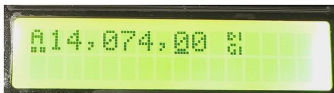
This means that QMX has been put into transmit mode via an appropriate CAT command, and that it is receiving audio from the PC; however the audio level is too low, so there is no RF.
