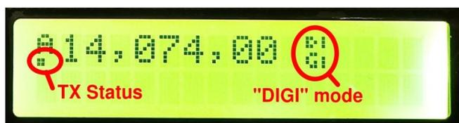
This means that QMX has been put into transmit mode via an appropriate CAT command from WSJT-X, however it is not receiving any audio, so there is no RF output. The usual reason for this is that QMX has not been selected correctly as the output device in the WSJT-X audio settings screen. Refer to the section above on the audio configuration. The single dot could also mean that there is no audio because somewhere in your PC sound settings you have MUTE enabled.
