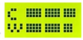
number of pixel columns is the number of dB of AGC attenuation divided by the "AGC db per bar" parameter.
