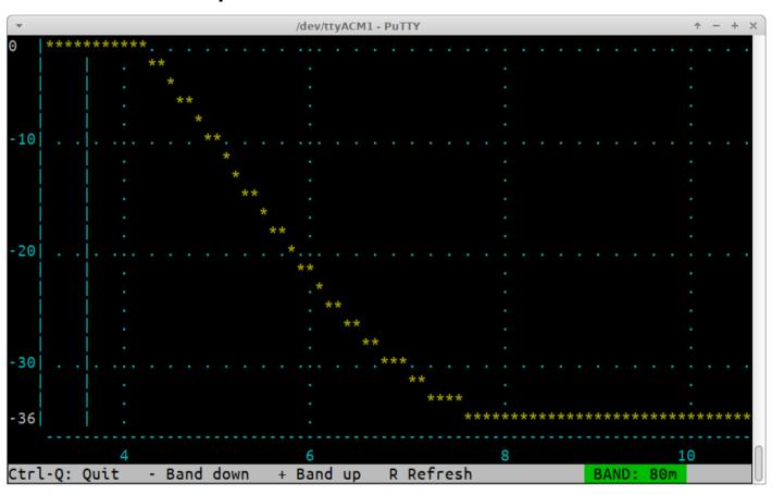
The LPF sweep tool transmits at ¼ of full power, and uses the Power/SWR bridge to measure the output power. To ensure accurate results a dummy load must be used at the output. The frequency range is set to run from the lower band edge frequency in the Band Configuration screen, to 3x the center frequency (the third harmonic frequency). The 0dB point is referenced to the signal level at the band center frequency.
