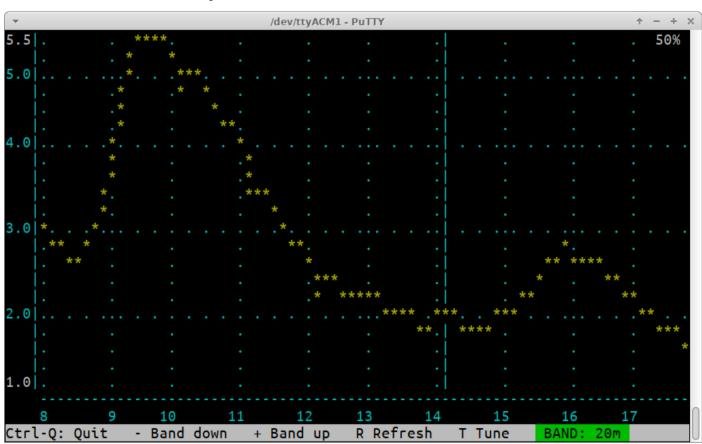
The SWR sweep tool has the same frequency range as the RF sweep tool; it displays the measured SWR at each frequency. During the sweep the PA voltage is set to a proportion of full power voltage determined by the "Tune %" parameter in the Protection menu. Remember that due to the square-law relationship between voltage and power, when the voltage is halved the power output is one quarter of full power. If the power is too low, the SWR measurement will be
