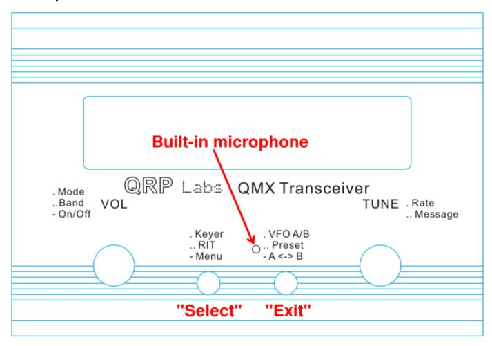
This diagram shows the operating controls of the QMX. There are two rotary encoders at left and right, and two push-buttons in the center. The main function of the left rotary encoder is Volume adjustment, and that of the right rotary encoder is Tuning. However, all of the controls have multiple functions, depending on the operating mode, menu editing, etc. The rotary encoders both have a button on their shaft activated by pressing the knobs, and these buttons also have multiple functions.
