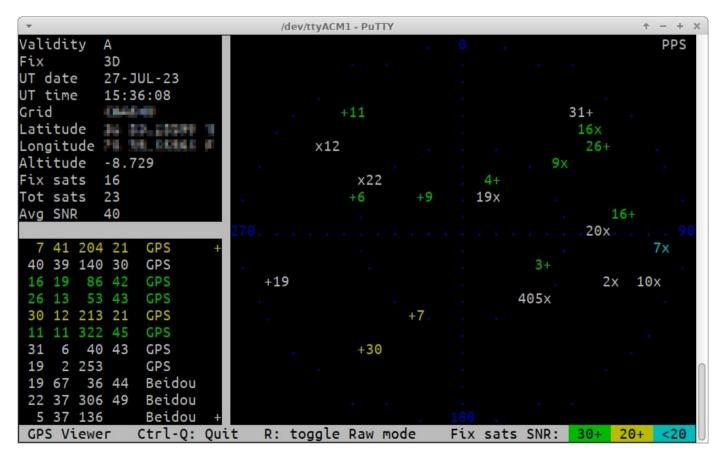
An example display is shown above. There are three panels: top left, some parsed information from the GPS data; bottom left: a list of all the satellites being tracked.
