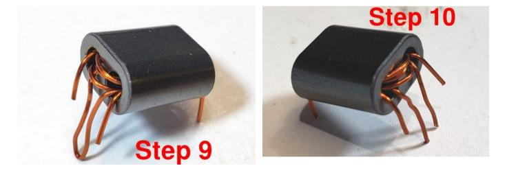
The transformer is now ready for installation in the PCB!
