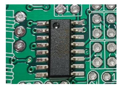
First solder two pins at diagonal opposites on the IC (above right). Then you can check to make sure that the chip is still nicely positioned on the PCB, and make any
