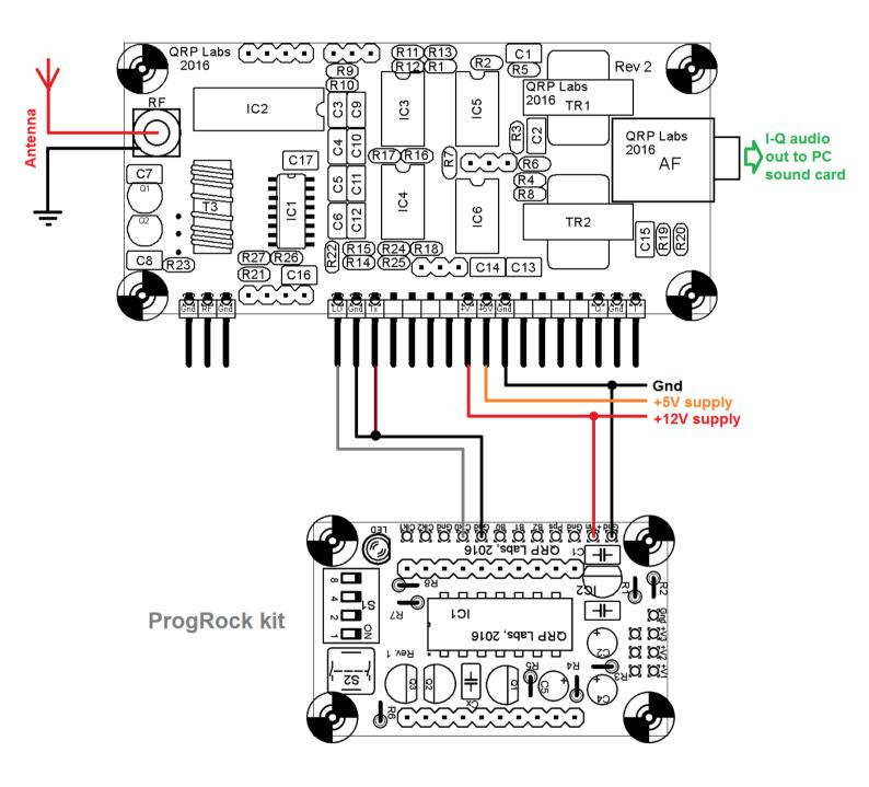
This example shows the VFO/SigGen kit used to provide a rotary-encoder tuned variable frequency LO for the receiver. The VFO/SigGen kit has a "Multiplier" setting which should be set to 4, so that the output frequency is 4x the displayed (reception) frequency.
