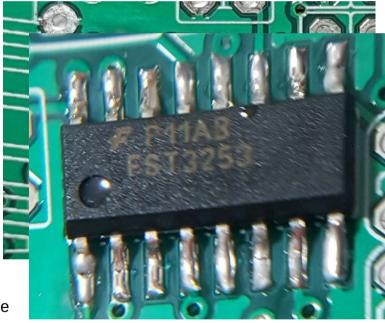
necessary corrections. When you are happy with the chip position, you can proceed to soldering the other pins. Pay particular attention to pin 8, which is connected to ground. Although the pad is connected to the groundplane with thin thermal traces, it will still tend to dissipate heat away from the joint, which can make it harder to get a good joint.
