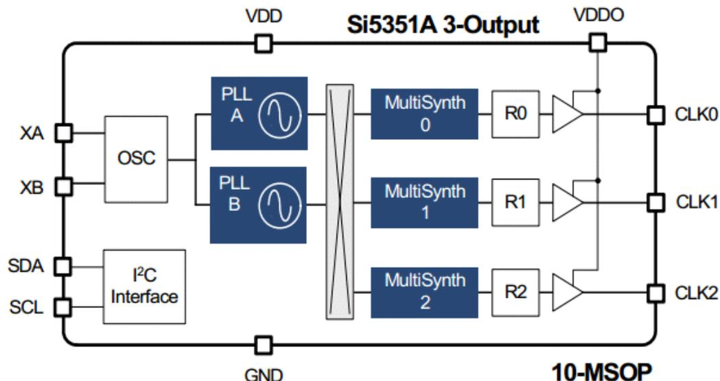
2200m (136kHz) to 2m (145MHz). A 25MHz crystal cannot provide WSPR tone spacing on the 2m band.
