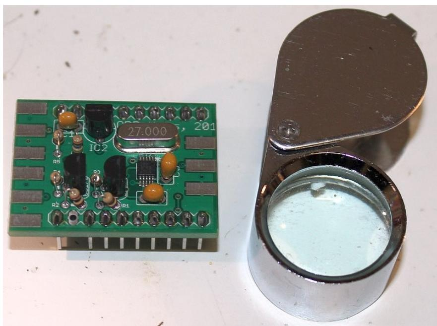
For those using the module in the Ultimate3 kit, make sure there is no pin soldered at pin 12. When using the module in the Ultimate3S kit, you can keep pin 12.
