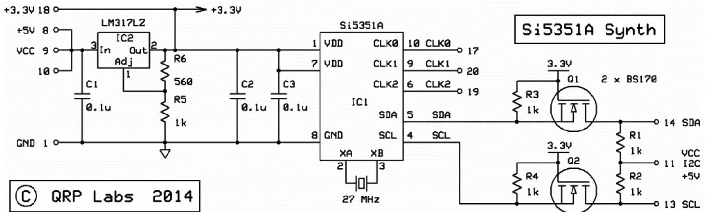
All module pins labeled "GND" are internally connected within the module. Similarly +5V pins (8, 9, 10) are also internally connected on the module PCB. Pin 11 is the pull-up resistor positive supply voltage for the level converters. For ordinary use, with a +5V I2C bus, pin 11 should be connected to +5V. The connection is provided separately (not connected to +5V internally) in case you wish to use a different I2C bus voltage.
