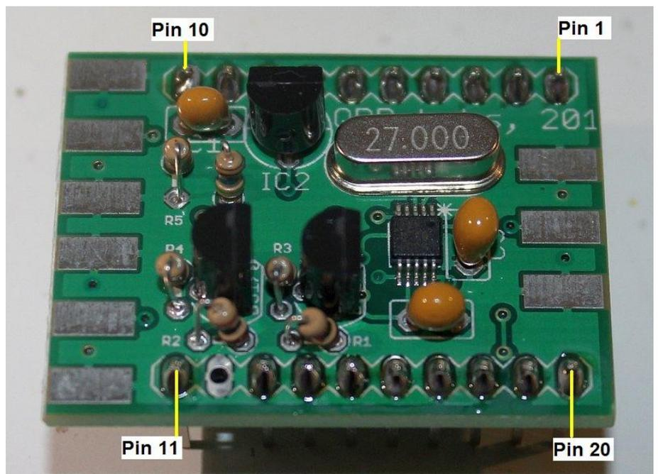
Note that in relating the pinout to the physical module, designated pin 1 is near the shorter PCB end of the module, as shown in this photograph. The photograph is an earlier PCB revision without the TXCO pad.
