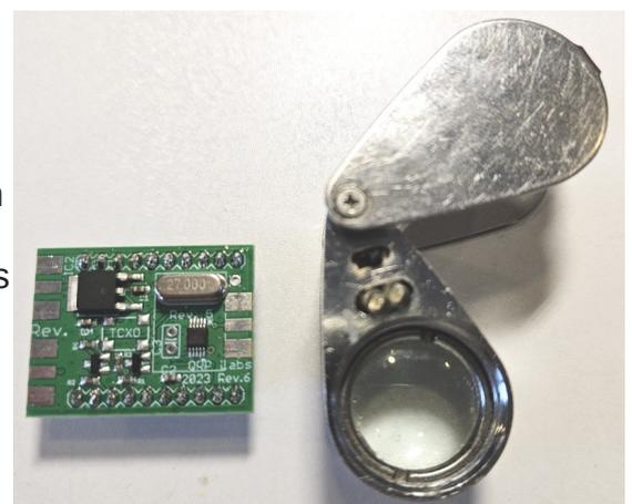
For those using the module in the older Ultimate3 kit (2014 and earlier), make sure there is no pin soldered at pin 12. When using the module in the Ultimate3S kit, you can keep pin 12.
