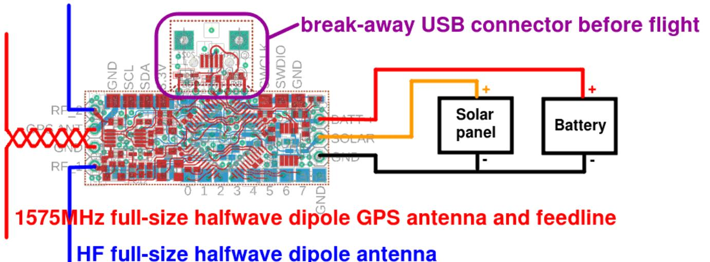
The HF antenna needs 1/4-wavelength on each leg (for example, each leg is 5m for 20m operation). A typical flight configuration has the top end of the top leg tied to the balloon, and the U4B payload suspended directly in the middle of the dipole.
