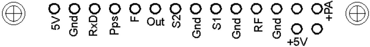
The diagram shows the connection pads along the edge of the board. The pin-spacing is 0.1-inches and a suitable connector could be used if desired. These are further described in the following sections. From left to right:
