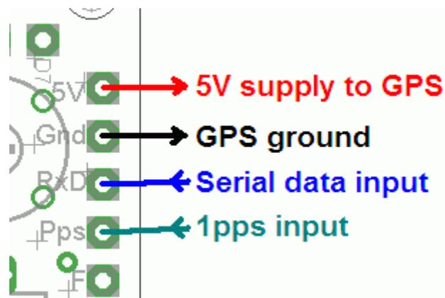
In cases where the location information is not required (modes other than WSPR) or you wish to enter it manually, the serial data input can be left unconnected. The 1 pps input is enough for the frequency lock function. Note that the frequency locking function can only operate if you have selected a wait period between message transmission (i.e. a non-zero “Frame” parameter).
