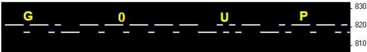
In Frequency Shift Keyed CW (FSK/CW) the dahs and dits have the same timing as traditional (slow) morse i.e. QRSS, but the carrier is always on and “key down” is indicated by a slight upwards shift of a few Hz. FSK/CW is the most popular of the slow-signal modes.
