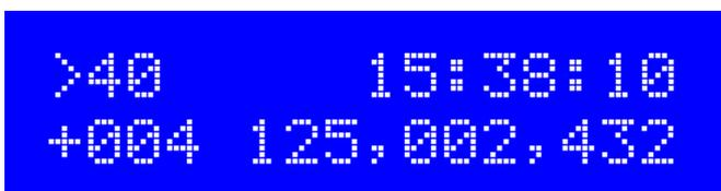
In this example, the calibration just completed has increased the reference clock value by +4Hz to 125,002,432Hz (Ultimate 3 in this example; Ultimate 3S will show a frequency near 27MHz).
