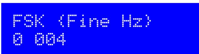
This configuration screens containing TWO settings relating to the way Frequency Shift Keying (FSK) is applied.
