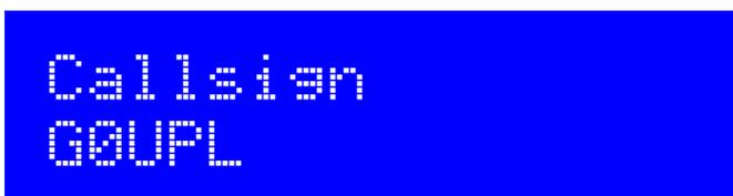
The callsign setting is an alphanumeric setting, which may be up to 14 characters long. It can theoretically include punctuation but clearly that isn't normally used in a callsign. The callsign is NOT used for the normal message transmission in most modes.
