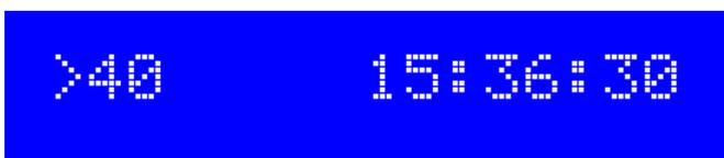
In this example, the time is 15:36:30 and the system is waiting until 40 minutes (time 15:40:00) to start the next message transmission. Additionally the heartbeat will flash, in the space on the top row. When a calibration is about to take place (GPS mode is non-zero) , there will be an additional second line display:
