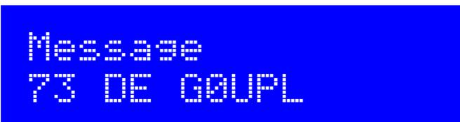
The message setting is an alphanumeric parameter which may be up to 250 characters long. For FSKCW, DFCW, CW, QRSS modes, it must be in the range A – Z, 0 – 9, / or a space character. Hell modes can use punctuation characters as well, but not the \* character.
