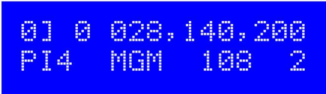
PI4 is a beacon mode with a 1-minute sequence. The transmission consists of:
