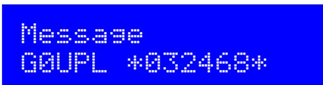
The callsign G0UPL is sent in ordinary FSK/CW with height and speed according to the configuration settings. Next comes a custom message, the duration of each symbol is 03 seconds. The shifts are 1, 2, 3, 4Hz respectively. On Argo, this message produces (with kit configuration FSK (Hz) = 04, Speed = 003):
