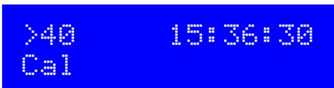
Once the actual frequency calibration starts, the Cal text is followed by a status bar which indicates the progress of the calibration. When calibration has completed, the new reference frequency value for 10 seconds (or whatever Cal Time is set to), as well as the change that was made since the previous calibration. For example:
