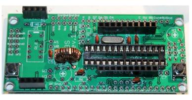
modules first; then use the Si5351A and LPF boards plugged into the sockets. You can then solder the pins, ensuring correct alignment.
