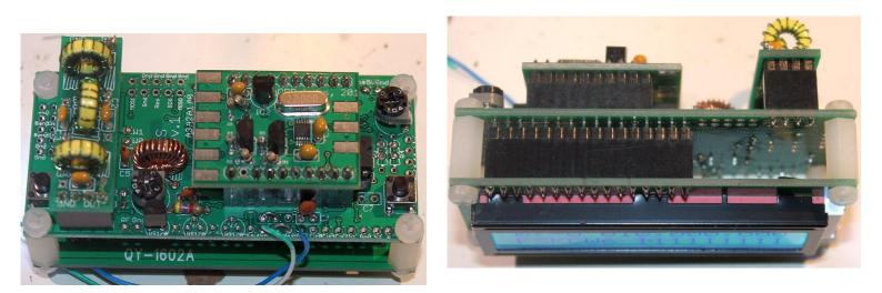
Ensure that the Si5351A synthesiser module is inserted the correct way round as shown in the photograph. The Low Pass Filter kit module should be plugged in with the "Out" legend aligned next to the RF Output connector of the main PCB (see photo).
