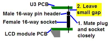
between the male header (plug) and the U3S PCB. I have found this method works successfully.
