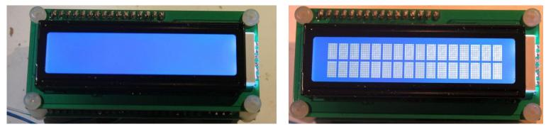
When you see "Diagnostic Mode" it means all is well with the processor and the LCD communication. When you press the left button, diagnostic mode will be cleared. Then you should see the flash screen. If the Si5351A module is correctly built and inserted, the firmware will recognise it. The text in the splash screen will say "Ultimate3S". The "S" is important, it signifies that the Si5351A has been correctly detected.
