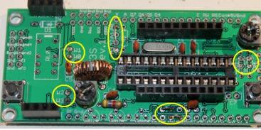
You may also install a jumper at the +PA and +5V connections at the bottom of the picture below, in order to power the power amplifier (PA) with the 5V supply. You should leave out this jumper if you intend to run the PA at a higher voltage. See more details in the "Hardware options" section below.
