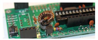
The transistors are located at the edge of the PCB with their flat side outwards. This is to allow easy attachment of a heatsink if desired (for higher voltage and hence higher power operation).
