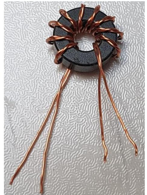
Now it's necessary to identify which wire belongs to which winding. The only way to do this is with a DVM as continuity tester. First, untwist and straighten the wire ends that are not wound around the toroidal core (above right).
