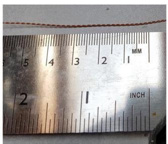
Now cut off the untidy pieces at one and, and the loop from the other: and this is the piece of wire that will be used to wind the FT37-43 toroidal core as a bifilar transformer.
