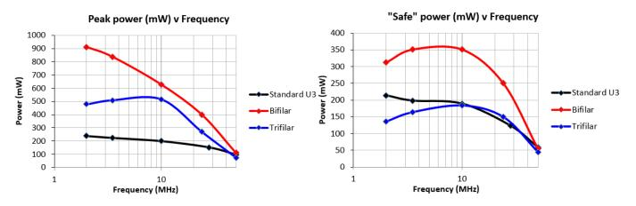
The bifilar option is recommended. Note, however that if you are planning to use the 5W HF PA kit with your Ultimate3S – then you should use the 25 turns single winding option, which works better with the 5W HF PA kit.
