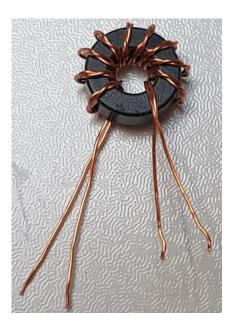
Now it's necessary to identify which wire belongs to which winding. The only way to do this is with a DVM as continuity tester. First, untwist and straighten the wire ends that are not wound around the toroidal core (above right).
