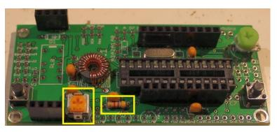
Please see section "PA bias set-up" below. The photograph (right) shows R5 in the mid position. In the correct completely ANTI-clockwise position, the "472" text will be to the right side, next to the Q1 position.
