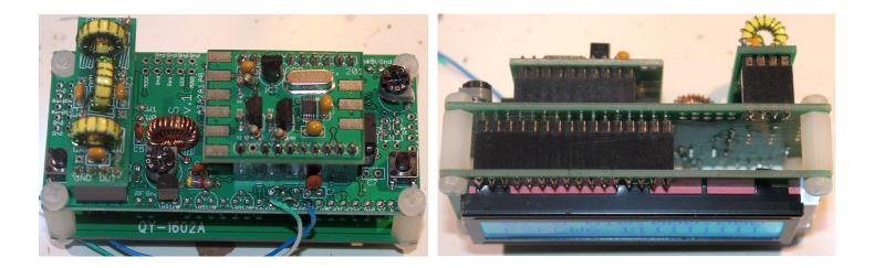
Ensure that the Si5351A synthesiser module is inserted the correct way round as shown in the photograph. The Low Pass Filter kit module should be plugged in with the "Out" legend aligned next to the RF Output connector of the main PCB (see photo).
