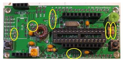
The wire jumpers can be made from offcuts from the other components e.g. capacitor leads. When installing these wire jumpers, I find it convenient to install them as a small semi-circular arch, perhaps 5mm high off the board. This is so that later, if they need to be removed (for different hardware options configuration), you can easily cut the links using wire cutters. It is easier than un-soldering them.
