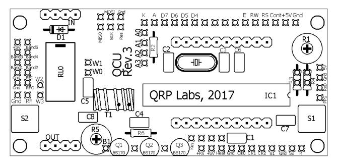
Pay special attention to the orientation of the semiconductors. For IC1, the dimple in the PCB silkscreen must be aligned with the dimple at the top of the IC socket and the IC.
