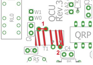
You must connect a bridge wire across both holes at the "1" end as shown. At the "2" end be sure to put the wire in the right-side hole next to the C4 capacitor. Leave the left of the two holes empty!
