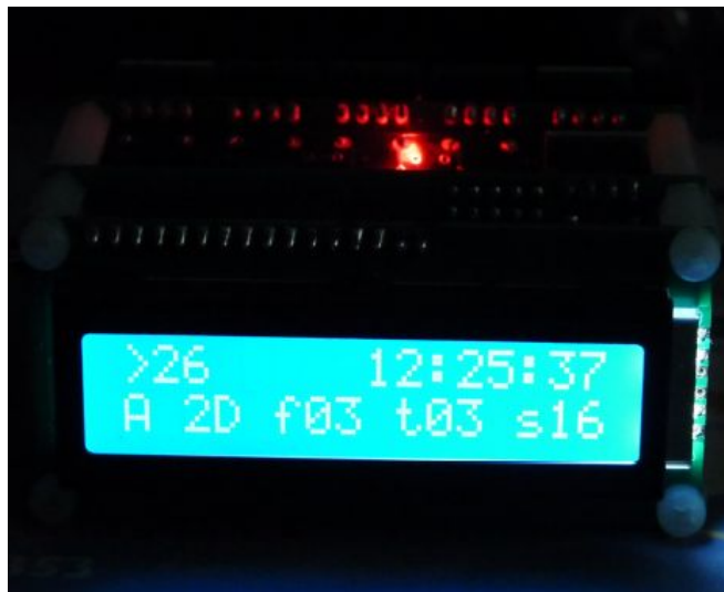
The Test U3 with 28MHz Carrier transmission from the signal source U3, the narrowest mode.
