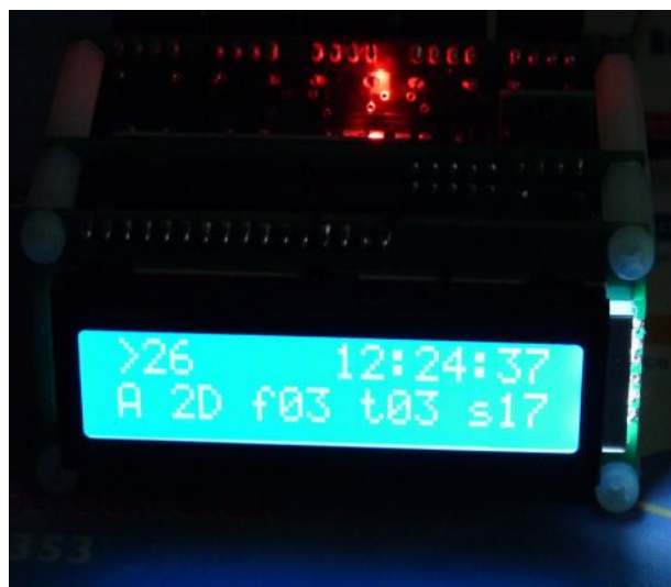
The Test U3 with 28MHz PI4 MGM transmission from the signal source U3. PI4 is a wide mode liable to produce sideband noise. Satellite numbers have dropped but is it due to TX noise.
