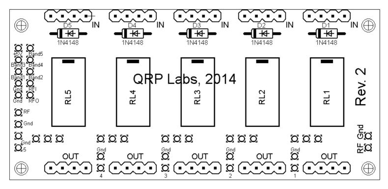
The order of construction is not important but a good principle to follow is to install the smaller components first, so that the larger ones do not prevent easy access.
