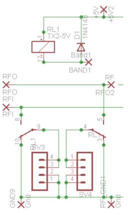
The relay-switched LPF kit can be used in your homebrew QRP transceiver project too. One side of the relay coils are connected to +5V. So to switch a relay, the appropriate band 1 to 5 input should be driven to a low voltage to energise the relay coil. A transistor could also be used to switch each relay coil.
