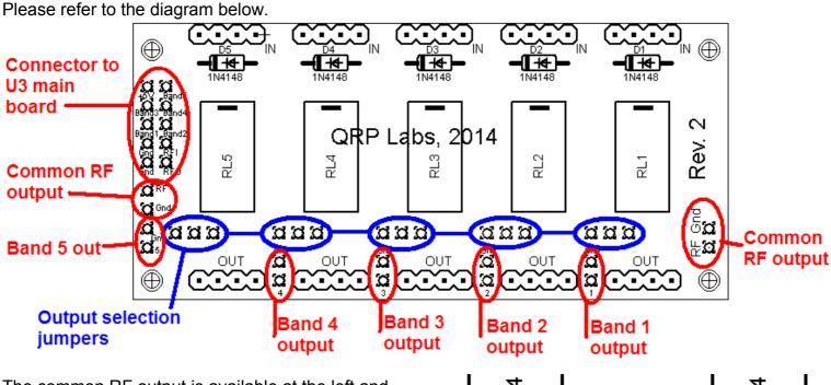
The common RF output is available at the left and right sides of the board. It is also connected to the Band 0 output, the output of the Band 0 relay on the main U3 board. Separate outputs Band 1 to Band 5 are indicated on the diagram. The output of each relay can be connected either to the common RF output, or to the corresponding individual band output.
