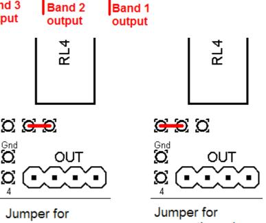
connecting relay output to the common RF out
