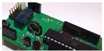
5) Fit the tall 10-way (5 x 2) pin header connector, pictured to the right, to the Ultimate3 PCB. The board photo (above right) shows the old (pre 6-Feb-2014 shipped kits) board interconnect method, using the standard-height header. Insert the tall header (right), with the short pins into the PCB, and the tall pins sticking up next to the relay.
