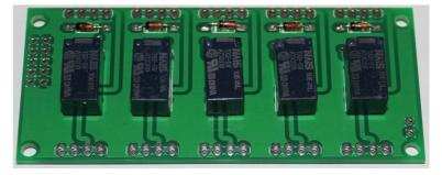
3) Fit and solder the ten 4-way sockets for the LPF's. Ensure that they are pushed in properly into the PCB, and at right-angles to the PCB. One way to do this, is to plug in a constructed LPF to ensure correct orientation of the sockets, then solder them to the PCB.
