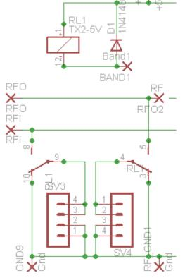
The relay-switched LPF kit can be used in your homebrew QRP transceiver project too. One side of the relay coils are connected to +5V. So to switch a relay, the appropriate band 1 to 5 input should be driven to a low voltage to energise the relay coil. A transistor could also be used to switch each relay coil.
