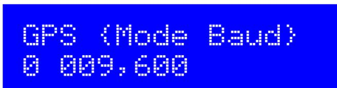
The first setting is the GPS mode. This controls how and whether GPS is used. If set to a non-zero value, and a GPS module is connected and producing a valid 1pps signal, then the accurate time pulses from the GPS unit will be used to discipline the output frequency(s) of the VFO/Signal Generator.
