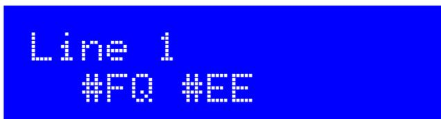
The Line 1 and Line 2 configuration settings determine the display format. Line 1 is the top row of the LCD, Line 2 is the bottom row. You can enter free fixed text (for example, your callsign). You can also include #tags. Each tag is a # character followed by a two-character identifier. Valid tags are replaced dynamically. Obviously the most useful tag to include is the #FQ tag, which displays the frequency on the display.
