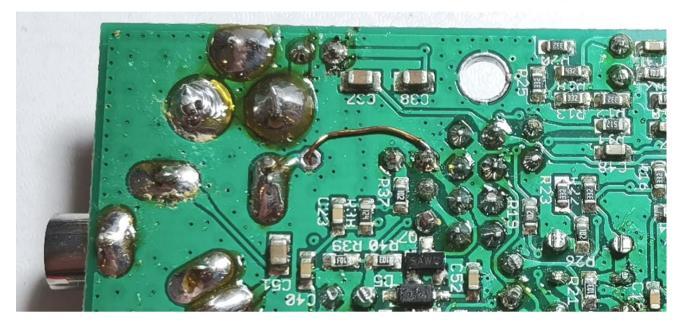
Finally, the connection that controls AGC ON/OFF, if you are installing it.
