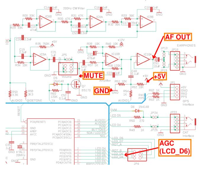
The AGC board fits snuggly in the area of the PCB shown in the diagram below. There is an outline of the AGC board footprint on the QCX+ PCB silkscreen.
