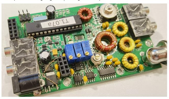
Firstly, the +5V connection must be made from the +5V pad of the AGC board, to the voltage regulator. Connect this wire to the center pin of the AMS1117-5.0 voltage regulator (as shown in the diagram on the preceding page, NOT the above photo which is a Rev 2 board).
