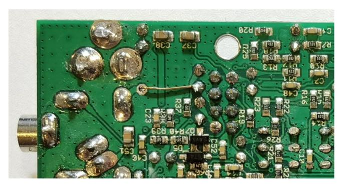
Finally, the connection that controls AGC ON/OFF, if you are installing it.
