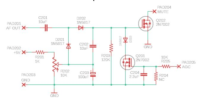
The AGC module schematic is shown above.
