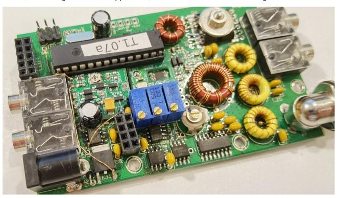
Firstly, the +5V connection must be made from the +5V pad of the AGC board, to the voltage regulator. Connect this wire to the rightmost pin of the 7805 voltage regulator (as shown in the photograph).
