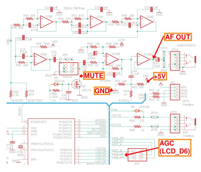
The AGC board needs a place to sit. An appropriate location where there is enough space, is on top of the "Labs" part of the QRP Labs logo, right in the middle of the QCX+ PCB. You can secure it to the PCB using double-sided tape or hot glue or some other type of glue. Before gluing it down, solder on five hookup wires for the five connections.
