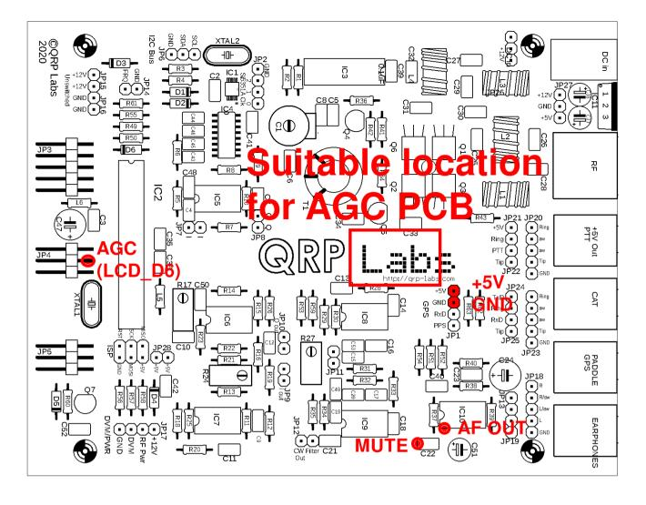
The five hookup wires should be soldered as follows. Refer to the photograph below.
