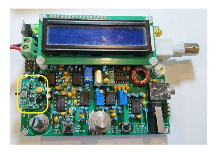
Before gluing it down, solder on five hookup wires for the five connections.
