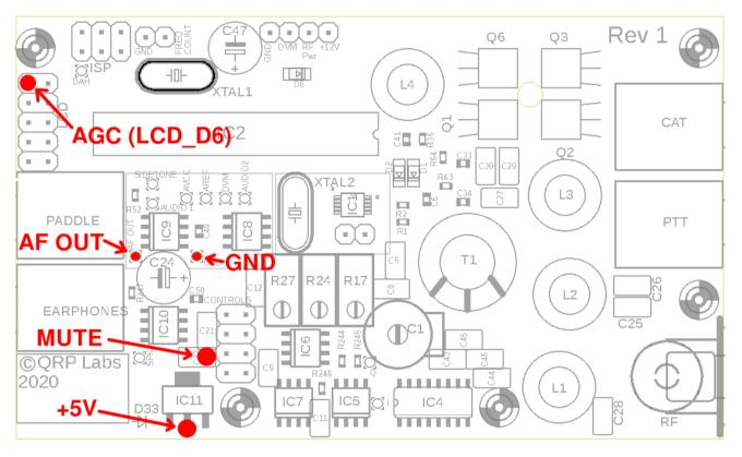
The "AF OUT" and "GND" connections are the easiest because the holes on the AGC board line up precisely with corresponding existing holes on the main QCX-mini PCB. These holes are the ones nearest to the 470uF capacitor, and are also identified by the yellow arrows in the photograph above.
