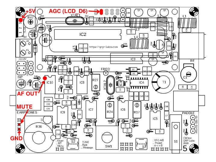
The five hookup wires should be soldered as follows. Refer to my diagram above.
