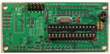
The wire jumpers can be made from offcuts from the other components e.g. capacitor leads. When installing these wire jumpers, I find it convenient to install them as a small semicircular arch, perhaps 5mm high off the board, as pictured. This is so that later, if they need to be removed (for different hardware options configuration), you can easily cut the links using wire cutters. It is easier than un-soldering them.
