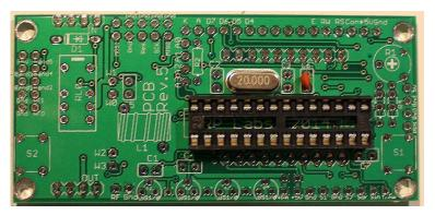
apparently they will work fine without any capacitors; the board and lead parasitic capacitances are sufficient for reliably operation. It does not matter that the oscillation frequency will not be exactly 20MHz, this is compensated in software.
