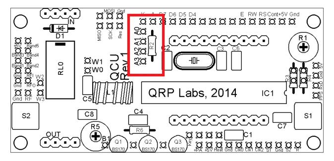
The LCD module has a blue LED backlight. The brightness of the LED can be set up using a jumper wire at the locations A0..A3, or optionally a resistor R2 which you may select for your preference. Choose one of the four options for the backlight as listed below.
