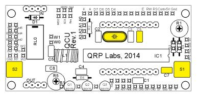
Note that the 22pF capacitors C2 and C3 either side of the crystal are NOT fitted – the 20MHz crystal has been found to oscillate reliably without them (there were some occasional issues when the 22pF capacitors were fitted). Therefore 22pF capacitors C2 and C3 are not supplied.
