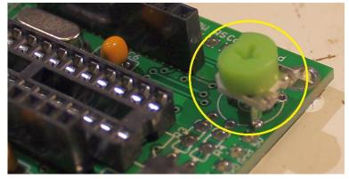
Adjust this potentiometer to the fully clockwise position initially.
