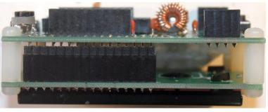
The combined 16-way plug and socket when mated together, have a height of a little under 12mm. Therefore it is necessary to have a gap somewhere.
