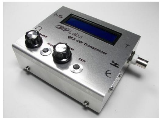
With the QSX design, I wanted to consider the enclosure right from the start. I wanted to avoid these subsequent enclosure headaches completely. Therefore, from the start, the mechanical design of QSX was chosen to permit easy mounting in an optional cut/drilled/silk-screen printed aluminium enclosure.
