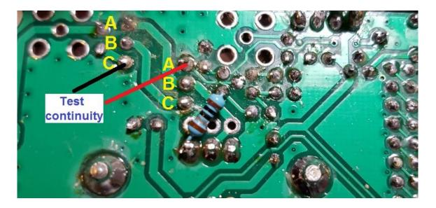
Note that this does NOT necessarily check that you correctly orientated the windings. The only way to do that, was with the DVM continuity check before inserting the transformer; and after identifying the windings, being careful not to mix the wires again while inserting the transformer in the PCB; finally checking again once the wires are inserted but before soldering.
