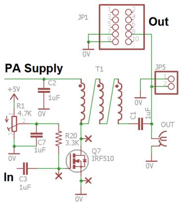
IRF510. The PCB has a second set of pads to suit the RD15HVF1.
