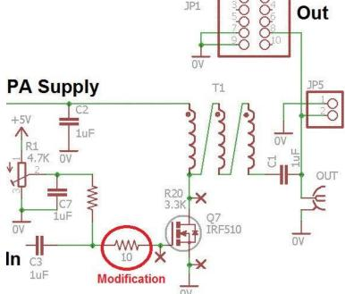
soldering a 10-ohm resistor on the bottom side of the PCB. The resistor location is shown in the above circuit diagram fragment which shows the IRF510 PA. The 10-ohm resistor is supplied in the kit and has colour code brown-black-black-silver-brown.
