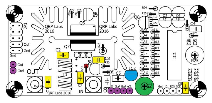
YELLOW: Capacitors C1, C2, C3, C7 and C8 are 1uF capacitors. The writing on the capacitor is "105". Be careful – the kit also contains one 1nF capacitor labelled "102" – do not mix them up!
