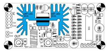
the heatsink mounting pins, then the transistor component leads themselves. A high wattage soldering iron may be needed for soldering the heatsink pins, as the heatsink will try to conduct away heat which may lower the temperature of the joint below the melting point of solder. You could leave the heatsink pins unsoldered if it seems troublesome. After soldering the transistor leads, cut off the excess lead length.
