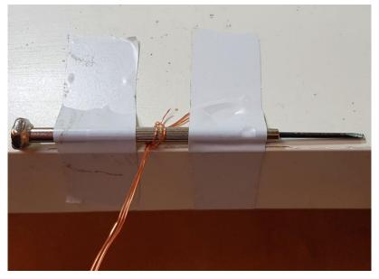
I put about 70-90 twists into a 25cm length of wire. The end result is something like the photo (right). The measurement scale is in cm.
