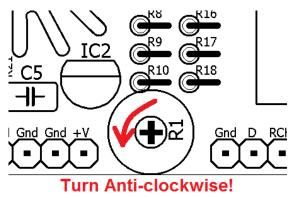
Theoretically the ideal bias point for the gate of the MOSFET, is where there is zero idle current through the IRF510 transistor, and where increasing the bias voltage any further would result in idle current starting to flow. This point has optimal power output, if the input signal amplitude is optimum, and it has best efficiency as well as spectral purity of the output. Of course in the real world, everything can (and does) change!
