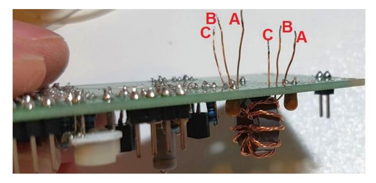
Now trim the wires underneath the board, and tin the ends again. The EASIEST way to do this is simply apply solder so that it sits in the hole and surrounds the 1mm of wire ending, and hold the soldering iron in that position for a few seconds until the enamel is burnt away. This tins the wires and solders them to the PCB pads.
