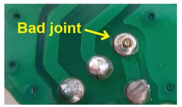
been held long enough on the joint. The enamel has not properly burnt off the wire, and there will be no electrical connection to the copper wire. The circuit will not work! So fix it!
