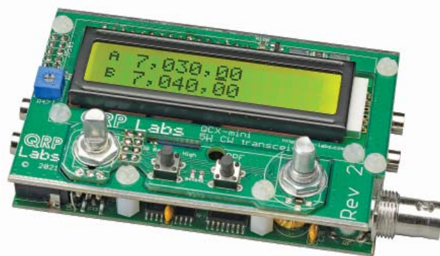
Figure 2 — The display/control PC board completes the sandwich, with the main board on the bottom.
