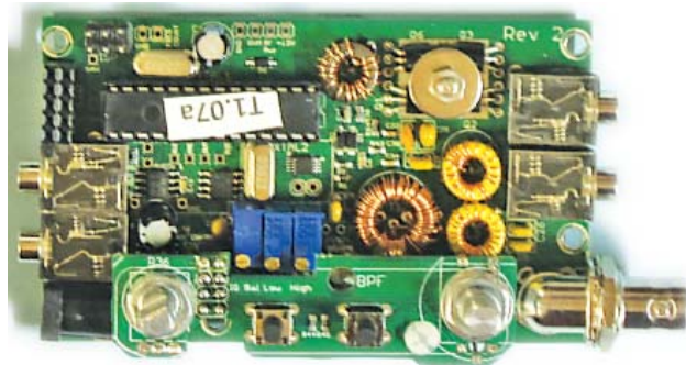
Figure 1 — The main circuit board carries most of the components for the receiver and transmitter sections. The microcontroller (white label) is at the upper left. T1 is the larger toroid near the center, and the socket that connects to the display board is in the upper left. The driver and final amplifier transistors are at the upper right, under the washer.
