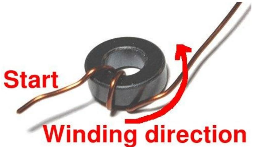
For all the toroidal inductors in the QDX kit, you will get it right, if you start as shown (photo, above right) and pass the wire through the toroid from the top side down through the hole, out and then around and over again; accumulating turns in the anticlockwise direction.
