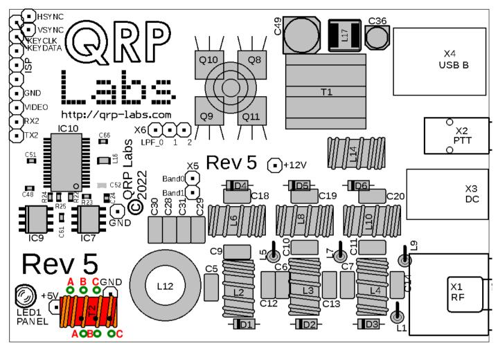
There are numerous SMD components in the vicinity so be VERY careful when soldering the wires of toroid T2, NOT to touch any of the nearby SMD components!
