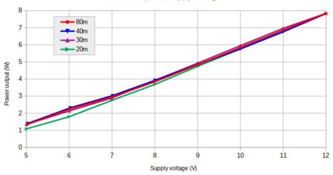
The following graph shows power output vs supply voltage for 40m operation, with the two alternative output transformer winding arrangements. 3:2 is less efficient but more suitable if you need to operate from a 12 - 13 V supply.
