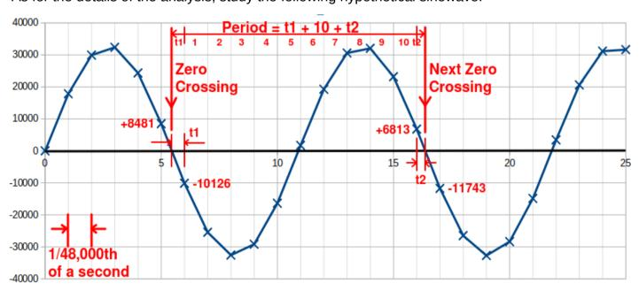
Remember that we have a built-in 24-bit 48ksps stereo USB sound card. Accordingly we get 48,000 samples per second. In this example I am assuming WSJT-X is used; WSJT-X outputs 16-bit samples, so the extent of the sinewave data is from -32,768 to + 32,767. The sound samples are received from the PC via the USB cable and are absolutely FREE of any noise. It's a lossless and zero noise transfer between the WSJT-X software on the PC, and the QDX's firmware. The
