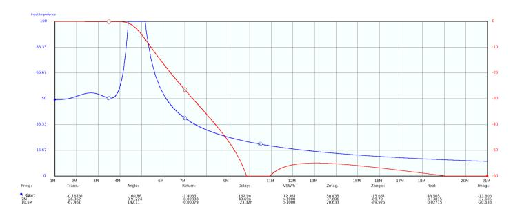
Fundamental: 3.5 MHz -0.17 dB Second harmonic: 7.0 MHz -26.4 dB Third harmonic: 10.5 MHz -67.5 dB
