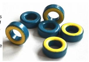
Winding the toroids as tightly as possible will slightly improve the performance of the Low Pass Filters. The following table lists the required number of turns, cut wire length, and inductance.
