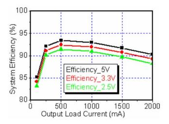
Figure 6-10. TPS562201  $V_{OUT}$  = 1.5 V Efficiency, L = 2.2  $\mu$ H
