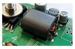
When the transformer is ready, insert the wires into the holes on the PCB, and continue with the installation steps listed here. For historical reasons the diagrams start at step 12... because the transformer winding instructions were moved to a separate document.
