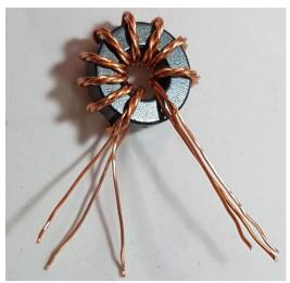
Now it's necessary to identify which wire belongs to which winding. You have three windings twisted together, they all use the same wire. The only way to do this is with a DMM as continuity tester. First, untwist and straighten the wire ends that are not wound around the toroidal core.
