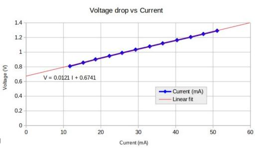
microcontroller code. It is also necessary to include the current contribution from the 1K resistors R1 and R6, which feed current on both receive AND transmit from the +5V bus. This current contribution is in the region of 4mA but again, varies depending on the total current since the voltage drop has current dependence as per the above discussion.
