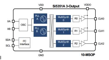
Voltage Controlled Oscillator in the range 600-900MHz (the PLL), then divided down to produce the final output frequency. The multiplication up and the division down are both fractional and so the frequency resolution is extremely finely controlled. The chip has two PLLs and three output divider units.
