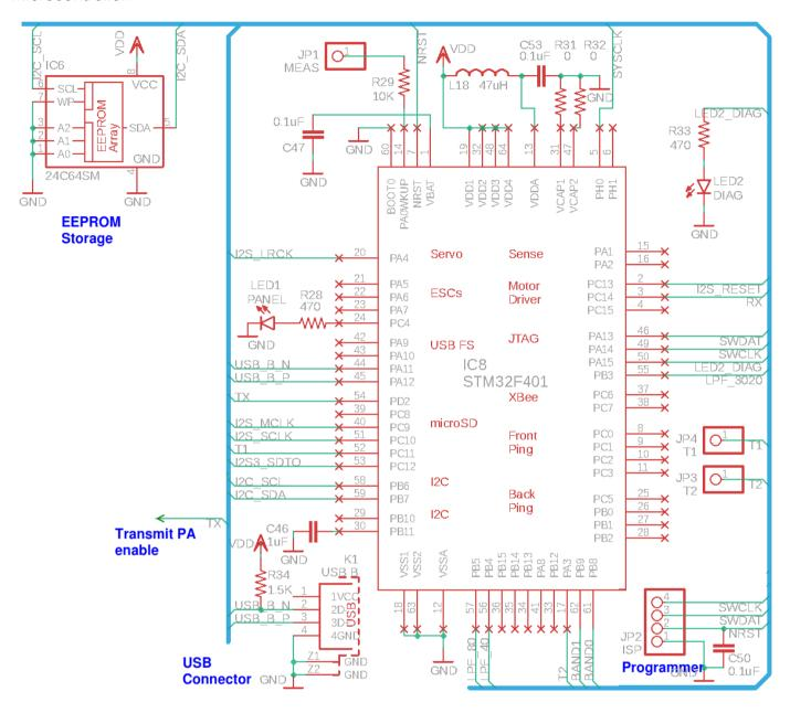
The microcontroller section of the schematic includes a 24C64 (8K x 8-bit) serial I2C EEPROM chip. Unlike the ATmega328 processors used in many other QRP Labs kits, the STM32 used here does not contain internal EEPROM so for storage of configuration parameters it is necessary to either use Flash storage or EEPROM. The problem with Flash storage is a limited 10,000 write-cycle specification which may be a little low. Therefore an external EEPROM chip is used.
