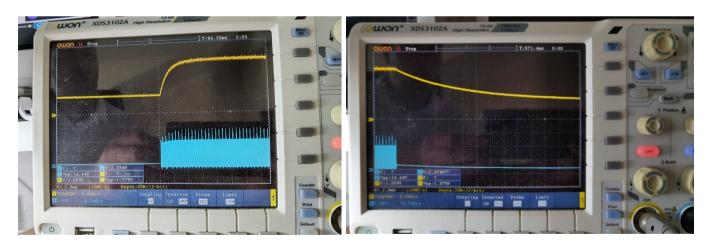
These two oscillscope photographs show switch-on (left) and switch off (right). The top (yellow) trace has a vertical scale of 500mV/div and shows the SMPS output voltage. The lower (blue) trace is here connected to the Q1 drain at 5V/div. Since the horizontal scale is 2ms/div, very much too slow to show the 100kHz switching waveform, the blue trace just shows here as a solid block.
