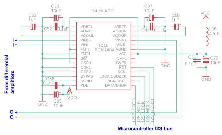
The PCM1804 Analog to Digital Converter (ADC) chip is a high performance stereo ADC chip with differential input. Its purpose is to convert the analog I and Q-channel signals to a digital representation to allow digital signal processing by the microcontroller, which implements a Software Defined Radio (SDR). The PCM1804 specifies a 112dB dynamic range and is used at 48 ksps (kilo samples per second).
