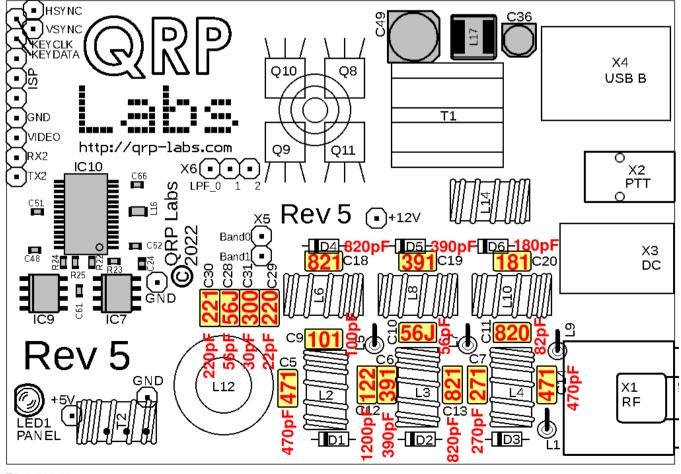
20 / 17 / 15 / 12 / 11 / 10m version: Install all 16 through-hole capacitors in accordance with the following diagram. The procedure is so easy that I have included all capacitors in a single assembly step rather than doing one diagram for each capacitor value. Nevertheless be very careful to insert the correct value capacitors in the correct places. Mistakes are hard to correct later.
