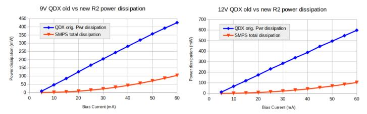
In a 12V QDX Rev 1 to 3a, according to the measurement data, R2 dissipates 387mW.
