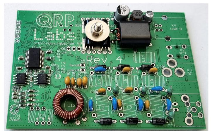
20 / 17 / 15 / 12 / 11 / 10m version: L12 is an inductor wound on a T50-6 toroid (yellow colour, large size), having several taps which are switched in according to the operating frequency (band). There are 20 turns in total, with taps at 11, 14 and 17 turns. The diagram shows the location of the taps at 11, 14 and 17 turns, which have larger holes, such that two wires can be inserted.
