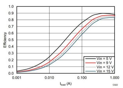
Figure 6-15. TPS562208  $V_{OUT}$  = 1.5 V Efficiency, L = 2.2  $\mu$ H
