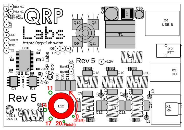
**Step 1**: Begin winding L12 as shown. Remember that in the nomenclature of toroidal inductors, each time the wire passes through the center of the toroid counts as 1 turn.
