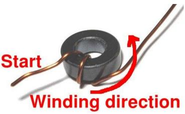
"winding direction". There are two directions you can wind the toroid. If you choose the right one, then all the wires will automatically end up near the holes they are to be soldered into. If you do it wrongly, it will be a bit messy.
