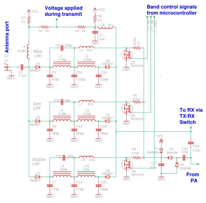
Very often relays are using for Low Pass Filter switching. However relays have several disadvantages:
