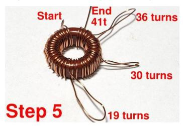
**Step 6**: Now with a pair of pliers, you can squeeze each of the loops into a sharp point, such that it is easy to fit through the large holes at the 19, 30 and 36-turn taps (see photo, right).
