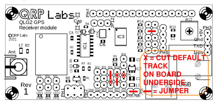
Connection of serial ports 1 and 2 (and also 3 if you have a pre-Rev 3 PCB) requires soldering wires directly to the microcontroller pins, a task to be undertaken with considerable care, to say the least.
