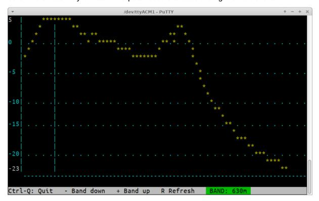
You also should run the Image sweep, to check the image rejection of the receiver. The results should be something like below. There will be quite a lot of variation in the image measurement but if you have an image rejection very low, such as -3, -4, -5dB etc., that will probably indicate a winding issue or installation issue with the T2 trifilar transformer, or perhaps a defective multiplexer IC in the quadrature sampling detector.
