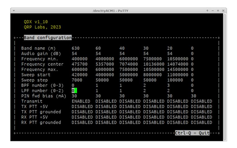
The BPF number, LPF number and PIN fwd bias cells have no meaning for the QDX-M because it is single band and there is no band switching. So you can ignore those. It is a very good idea to set the "Transmit" cells for all the other listed bands to "DISABLED" to prevent any accidental mishaps trying to transmit at incorrect frequencies into the 630m Low Pass Filter of your QDX-M.
