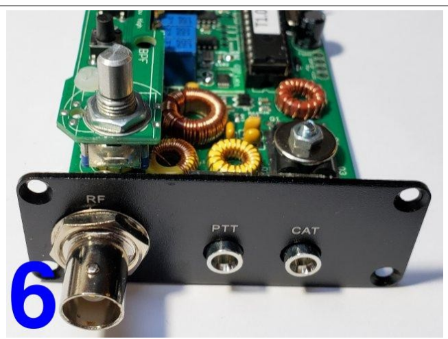
Bolt the right-hand side panel to the main PCB using the supplied BNC washer and nut
